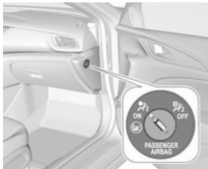
The front passenger airbag system can be deactivated via a key-operated switch on the passenger side of the instrument panel.
