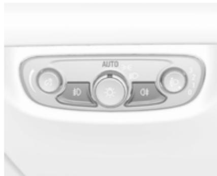
**AUTO** : automatic light control switches automatically between daytime running light and headlight
