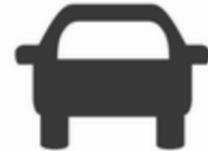
The green illuminated vehicle ahead control indicator
