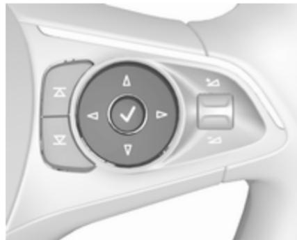
Press ◀ or ▶ to switch between the main menus or to return from a submenu to the next higher menu level.
