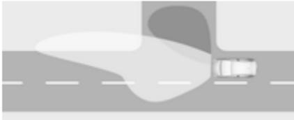
When turning off, depending on the steering angle and the turn signal light, particular LEDs are triggered which illuminate the direction of travel. It is activated up to a speed of 40 km/h.
