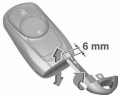
2. Insert the key blade again for approx. 6 mm and turn the key to open the housing. Further insertion of the key blade can damage the housing.
