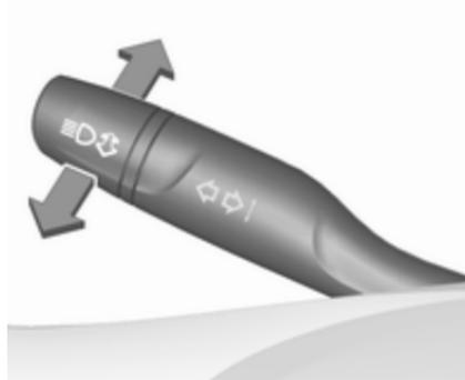
Push lever to switch from low to high beam.
