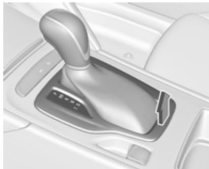
2. Release the selector lever trim from the centre console. Poke with a finger into the leather socket below the selector lever and push the trim upwards. Rotate trim to the left.
