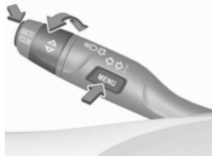
Press **MENU** to switch between the main menus or to return from a submenu to the next higher menu level.
