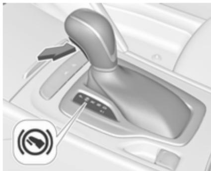
The selector lever is locked in **P** and can only be moved when the ignition is on, the release button on the selector lever is pushed and the brake pedal is applied.
