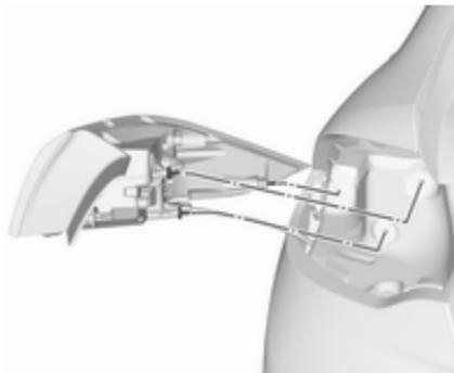
3. Carefully withdraw tail lamp assembly from recess and remove.
