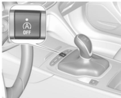
Deactivate the stop-start system manually by pressing
