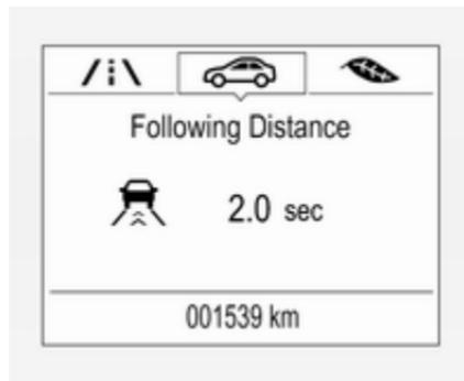
On Mid- and Uplevel display, select **Info** menu via steering wheel buttons and press **V** to select following distance indication ⇨ 104.
