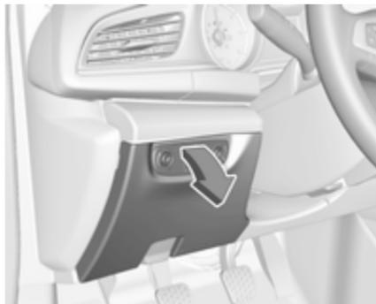
In left-hand drive vehicles, the fuse box is behind a cover in the instrument panel.
