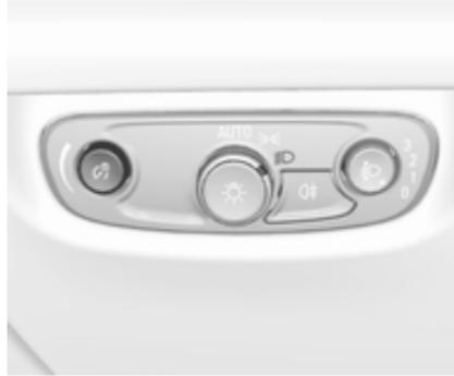
Brightness of the following lights can be adjusted in position **AUTO** when the light sensor detects night conditions, or in position
