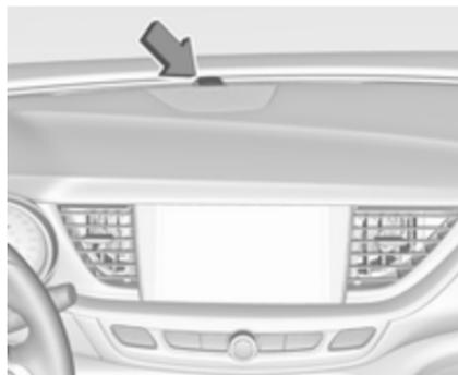
Status LED is integrated in the sensor on top of the instrument panel.
