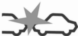
When the time to a potential collision with a vehicle in front gets too small and a collision is imminent, the collision alert symbol pops-up in the Driver Information Centre and the driver gets notified by a flashing red LED stripe or the pop-up symbol in the head-up display which is projected on the windscreen in the driver's field of view.
