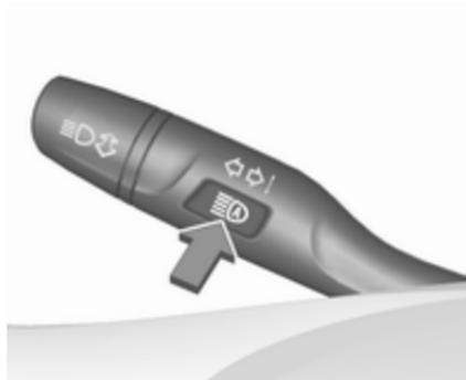
The green control indicator
