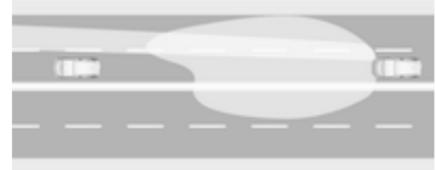
High beam assist includes a special motorway mode. When driving faster than 115 km/h on motorways, the light beam becomes smaller to avoid dazzling of oncoming traffic. When following vehicles ahead or passing, mirror dazzling for these vehicles is reduced.
