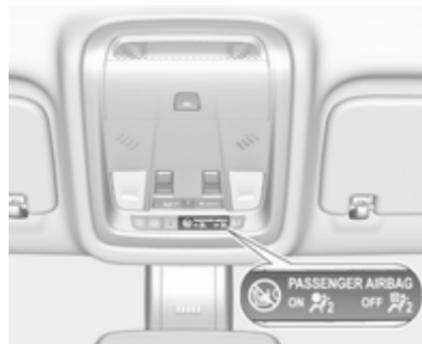
If the control indicator
