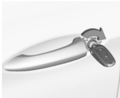
Push inside locking knob of all doors except driver's door or press
