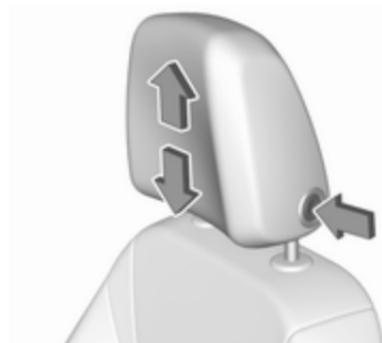
Press release button, adjust height, engage.
