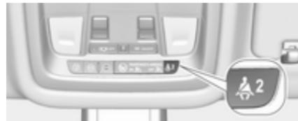
⚠ for front passenger seat illuminates or flashes red in the roof console, when seat is occupied.
