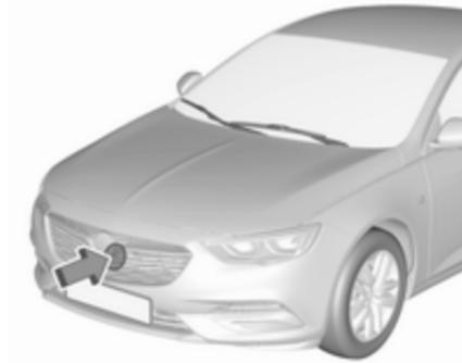
The radar unit is mounted behind the radiator grille behind or below the brand emblem.
