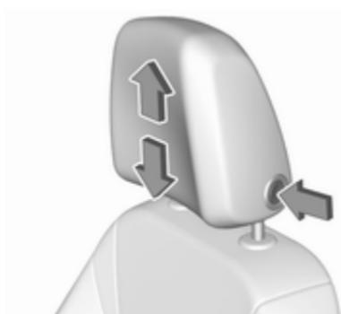
Press release button, adjust height, engage.
