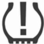
A detected low tyre pressure condition is indicated by the control indicator (⚠) ⇨ 101.
