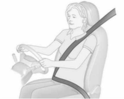
The seat belts are locked during heavy acceleration or deceleration of the vehicle, holding the occupants in the seat position. Thereby the risk of injury is considerably reduced.
