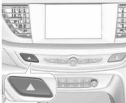
In the event of an accident with airbag deployment, the hazard warning flashers are activated automatically.
