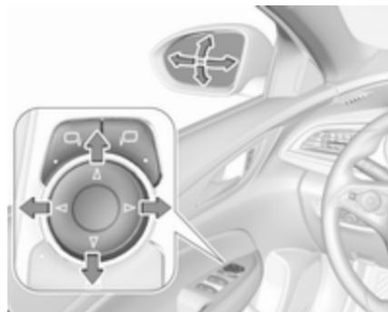
Select the relevant exterior mirror by pushing
