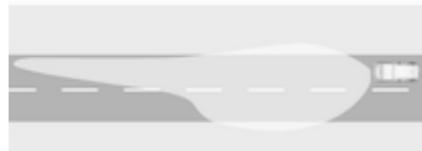
Activated automatically at a speed above approx. 55 km/h when driving in rural areas. The illumination of the current lane and the side of the road is improved. Oncoming and preceding vehicles are not dazzled.
