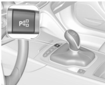
When searching for a parking slot, the system is ready to operate with a short press of **P** with a square symbol.
