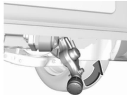
With the flat of the hand, swivel the released coupling ball bar to the right until it engages under the floor. Make sure that the release handle is back in its hidden initial position, otherwise the buzzing tone will not stop.
