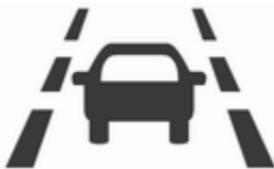
When the control indicator
