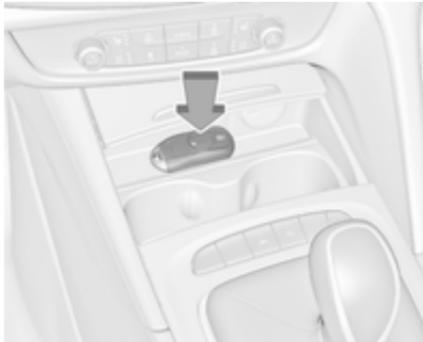
Open the cover of the centre console in front of the gear shift lever. Place the electronic key across with buttons upside in the transmitter pocket beside the power outlet, as shown in the illustration.
