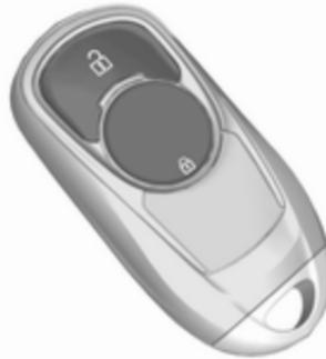
The central locking system can also be operated with the buttons on the electronic key.
