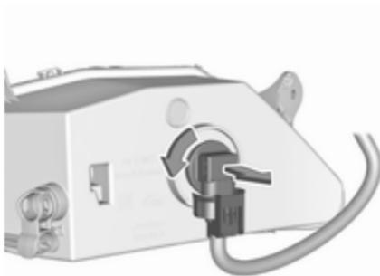
4. Turn the bulb socket anticlockwise and remove it from the light assembly.
