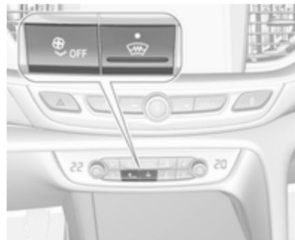
If the vehicle is equipped with heated windscreen, button **ON/OFF** is replaced by button
