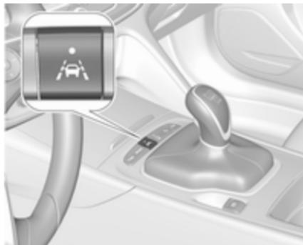
The lane keep assist is activated by pressing
