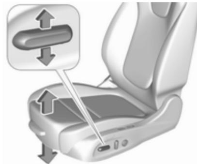
Move switch upwards/downwards.
