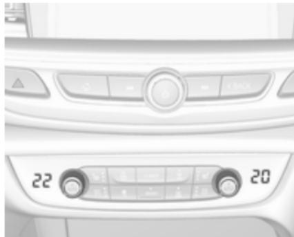
Set the preselected temperatures separately for driver and front passenger to the desired value using the left and right control dials. The knob on the passenger side changes the temperature for the passenger side. The knob on the driver's side changes the temperature for the driver's side or for both sides depending on activation of synchronisation **SYNC**. Recommended temperature is 22 °C. Temperature is indicated in displays beside the control dials and as pop-up in the Info-Display.
