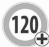
Additionally, the currently valid speed limit is displayed permanently in the lower line of the Driver Information Centre. In case a speed limit with add on sign is available, a + symbol is displayed in this area.
