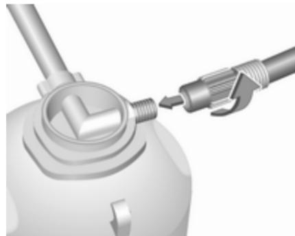
2. **Type 1:** screw the compressor air hose to the connection on the sealant bottle and fit the sealant bottle into the retainer on the compressor.
