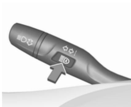
Activate high beam assist by pressing
