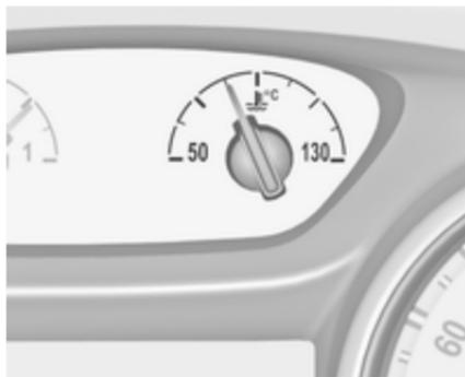
Displays the coolant temperature.
