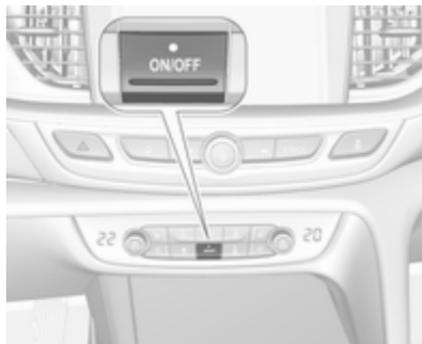
Cooling, fan and automatic mode can be switched off by pressing **ON/OFF**. When the system is deactivated, the LED in the button **ON/OFF** is not illuminated.
