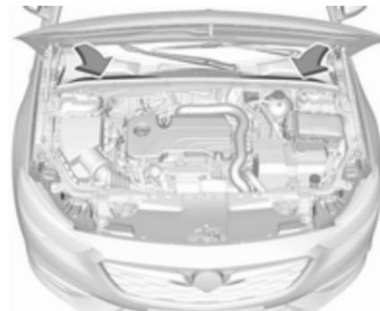
The air intake in front of the windscreen in the engine compartment must be kept clear to allow air intake. Remove any leaves, dirt or snow.
