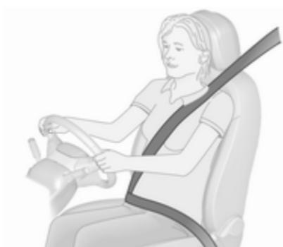
Pull out the seat belt and fasten in belt buckle. The seat belt must not be twisted and must fit close against the body. The backrest must not be tilted back too far (maximum approx. 25°).
