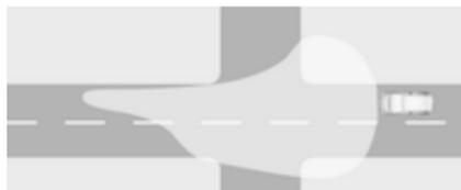
Activated automatically at a speed up to approx. 55 km/h and in situations with exterior ambient light. The light is wide and symmetrical. A special beam pattern is designed to avoid glare for other road users.
