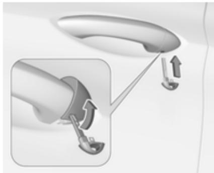
**Electronic key:** to remove the cap, press button at the back and extract the key blade from the housing. Insert the key into the recess at the bottom of the cap and swivel the key upward.
