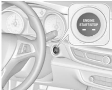
Electronic key must be inside the vehicle.
