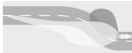
Particular LEDs, based on steering angle and speed, are additionally triggered to improve lighting in curves. This function is activated at speeds from 40 km/h to 70 km/h and reacts to steering angle.
