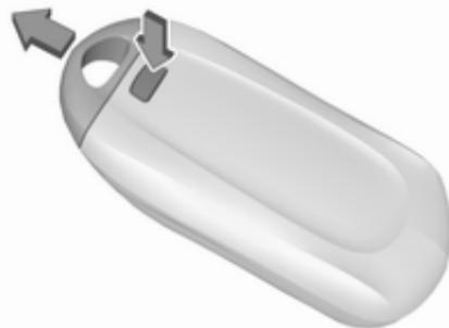
1. Press button at the back of the electronic key unit and extract the key blade from the housing.
