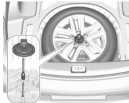
1. Stick the extension bolt onto the thread bolt.
