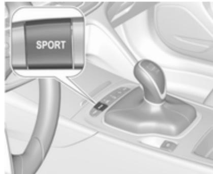
On vehicles with Flex Ride driving modes, the driver can slightly increase the Adaptive cruise control acceleration when Sport mode is selected.
