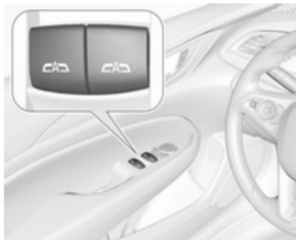
Operate **C** or **D** for the respective window by pushing to open or pulling to close.
