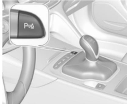
Press parking assist button **P**▲ to deactivate, the LED in the button extinguishes.
