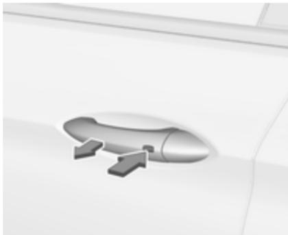
Press the button on the respective exterior door handle and pull the handle.
