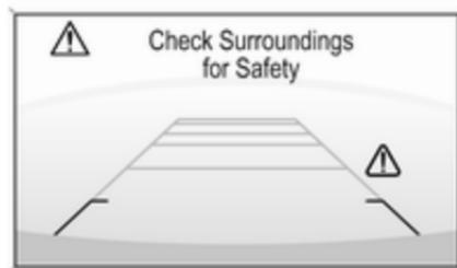
The area displayed by the camera is limited. The distance of the image that appears on the display differs from the actual distance.
