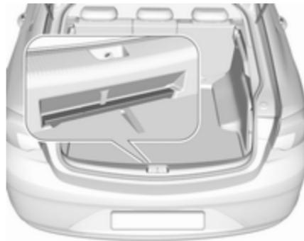
Stow the warning triangle in the space at the rear of the load compartment.
