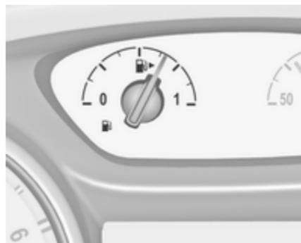
Displays the level in the fuel tank. The arrow indicates the vehicle side where the fuel filler flap is located.
