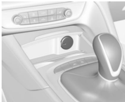
A 12 Volt power outlet is located in the centre console.
