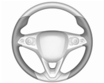
The recommended grip areas of the steering wheel are heated quicker and to a higher temperature than the other areas.
