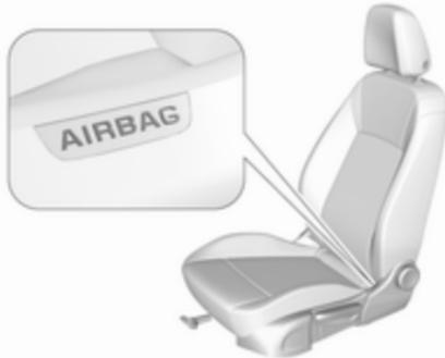
The side airbag system consists of an airbag in each front seat backrest and in the rear outboard seat backrests. This can be identified by the word **AIRBAG**.
