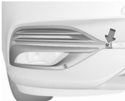
2. Undo screw and remove the faceplate.
