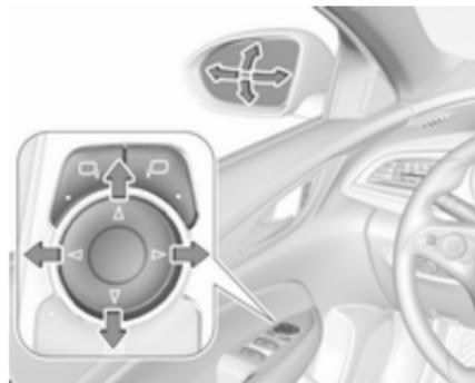
Select the relevant exterior mirror by pushing left or right mirror button. LED in button indicates the selection. Then swivel the control to adjust the mirror.
