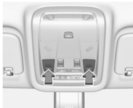
Operated by pressing the respective reading light.
