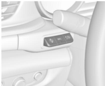
There are three controls above the light switch to operate the Head-up display.
