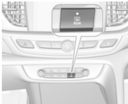
Operated by pressing
