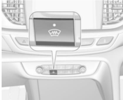
If the vehicle is equipped with heated windscreen, button
