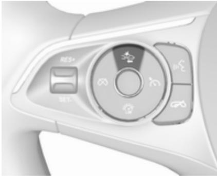
The first button press shows the current setting on the Driver Information Centre. Additional button presses will change this setting. The chosen setting will remain until it is changed. The alert timing will vary based on vehicle speed. The faster the vehicle speed, the farther away the alert will occur. Consider traffic and weather conditions when selecting the alert timing.
