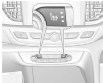
Adjust heating to the desired setting by pressing
