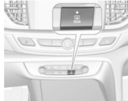
Operated by pressing
