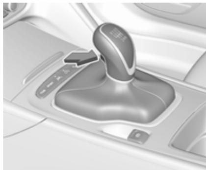
Reverse: with the vehicle stationary, depress clutch pedal, press the release button on the selector lever and engage the gear.
