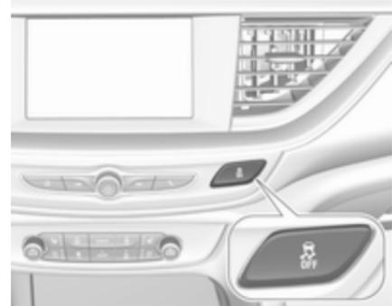
TC can be switched off when spinning of drive wheels is required: press
