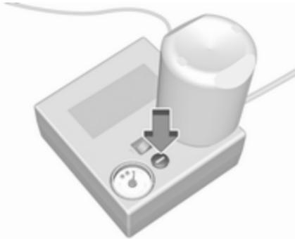
If the pressure is obtained within 10 minutes, correct to the prescribed tyre pressure by using the compressor to increase or
