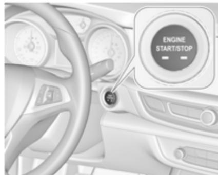
Power button: press **Engine Start/Stop** and release.
