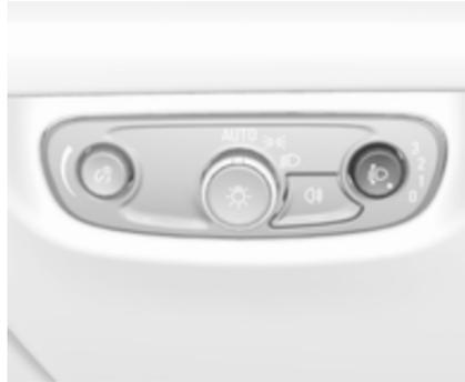
To adapt headlight range to the vehicle load to prevent dazzling: push and then turn  $\text{D}$  to required position.
