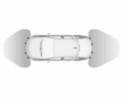
The system has four ultrasonic parking sensors each in the rear and front bumper.
