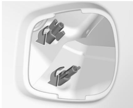
2. Unscrew the two plastic securing nuts from the inside by hand.
