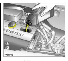
The amount filled must be between the MIN and MAX marks  $\diamondsuit$  230.
