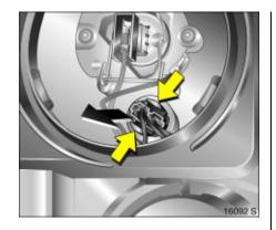
Push side lugs of parking lamp holder together and remove holder from reflector.
