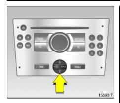
To select with four-way button Select menu items via menus and with the buttons/four-way button of the Infotainment system.
