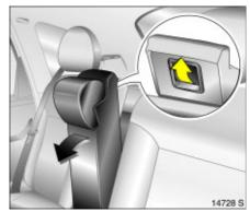
Fold the centre seat forward and lower. House centre seat belt in the holder in the ceiling  $\diamondsuit$  63.
