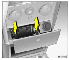
To empty, grip both sides of the ashtray insert at the spots illustrated and pull upwards.
