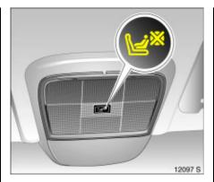
Vehicles with seat occupancy recognition can also be recognised by control indicator ⊌\*. If control indicator ⊌\* illuminates for approx. 4 seconds after the ignition is switched on, the vehicle is equipped with seat occupancy recognition ▷ 72.
