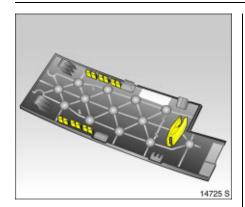
Keep spare fuses in the fuse box lid (shown in yellow in the Fig.). Open lid  $\diamondsuit$  182.
