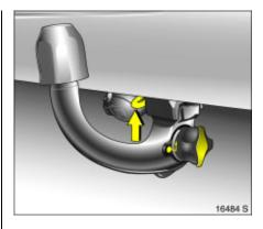
Lock the coupling ball bar in position by turning key to position 2 ₺ 159, Fig. 12416 T. Remove the key and press the protective flap into place.
