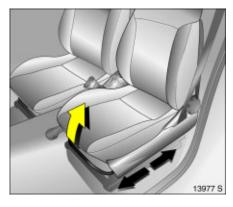
To adjust front seat leg room: Pull handle, slide seat, release handle Seats  $\diamondsuit$  44, Seat position  $\diamondsuit$  45.
