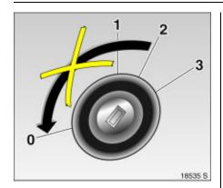
We recommend not stopping driving during cleaning, and not switching off the ignition. Cleaning is fastest at high engine revs and high loads.
