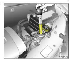
Have the concentration of the radiator contents tested by a workshop before winter starts. The amount of antifreeze must provide protection down to approx. -28  $\square$ C. A lower antifreeze concentration will reduce the amount of protection from frost and corrosion. Add
