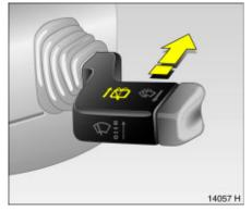
**Rear window washer and wiper system**Push stalk forwards. The rear window wiper wipes in timed interval mode. Switch off by pulling stalk towards the steering wheel.
