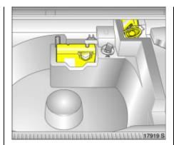
The tyre repair kit is in the stowage compartment beneath the floor cover in the luggage compartment.
