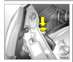
In vehicles with headlamp washing system \* Opening for refilling is in engine compartment behind the right-hand headlamp.
