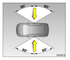
The side airbag system will be triggered:
