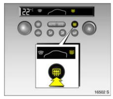
On vehicles with electronic climate control IIII appears on the climate control display.
