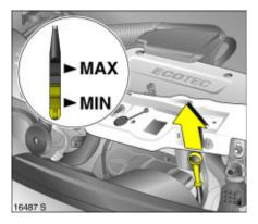
Check with the vehicle on a level surface. The engine must be at operating temperature and switched off for at least 5 minutes.
