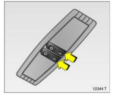
Courtesy lamps and rear reading lamps \* Centre switch position: The rear courtesy lamp comes on together with the front one when a door is opened.
