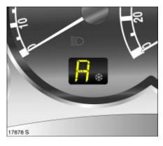
**Transmission display**Shows the mode and current gear.
