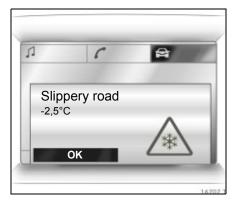
In vehicles with graphical information display \* or colour information display \*, a warning message **Slippery road** appears on the display as a warning for icy road surfaces. There is no message below -5 □C.
