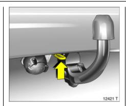
Eye for break-away stopping cable In the case of trailers/caravans with brakes, attach breakaway stopping cable to eye.
