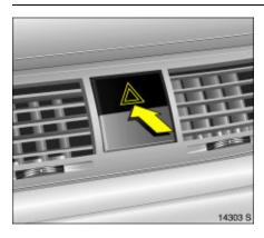
Hazard warning flashers Operated with the <u>&</u> button. Hazard warning lamps \$ 104.
