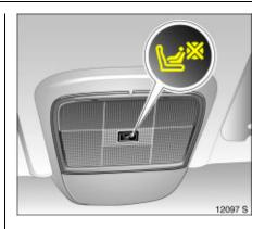
If the control indicator does not come on while driving, the front and side airbags for the passenger are not de-activated and there is a risk of injury or death to the child. Fit child restraint systems on the rear seat. Have the cause of the fault eliminated by a workshop.
