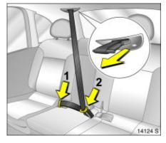
Three-point seat belt on centre rear seat Pull latch plates out of belt retainer in roof.
