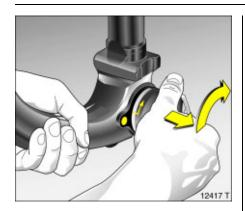
Otherwise, the coupling ball bar must be tensioned before it is inserted into the coupling housing:
