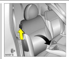
Fold down passenger seat backrest  $\*$  Push head restraint all the way down or remove  $\$\diamondsuit$  3,  $\$\diamondsuit$  46.
