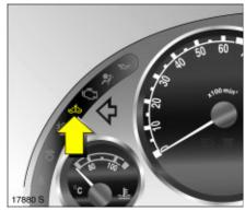
Control indicator for immobilizer औ> Control indicator औ> illuminates briefly when the ignition is switched on.
