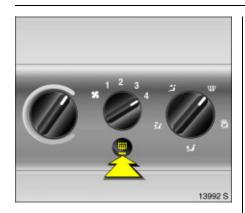
Heated rear window **\***Heating is activated or deactivated by pressing the ₩ button.
