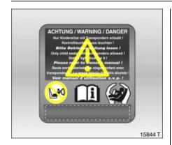
Vehicles with seat occupancy recognition can be identified by the sticker on the front passenger seat or on the side of the instrument panel.
