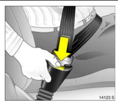
**Removing the belt**To release seat belt, press red button on belt buckle.
