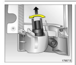
Fog tail lamp bulb: Rotate bulb mounting anticlockwise and disengage. Remove bulb from holder.
