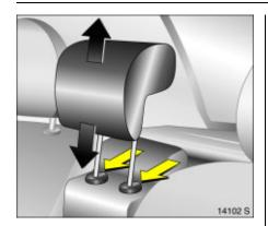
Adjusting the rear centre head restraint Pull head restraint upwards, press springs and push head restraint down.
