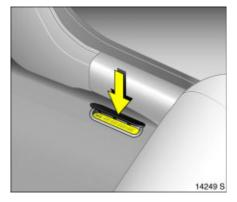
The vehicle identification number is stamped on the identification plate and on the right side of the floor of the vehicle under a cover between the front door and the seat.
