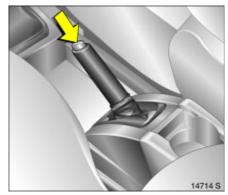
Releasing the hand brake: Raise lever slightly, Press release button, Lower lever fully Hand brake \$ 153.
