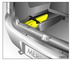
To open, remove the luggage compartment cover  $\clubsuit\, \diamondsuit\, 55,$  lift the floor using the handle and raise toward the front.
