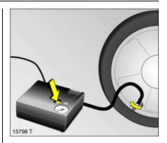
If tyre pressure is more than 1.3 bar, adjust to the prescribed value. Repeat the procedure until there is no more pressure loss.
