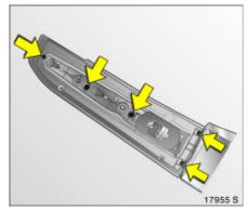
Slacken both screws on the back of the main bulb mounting. Press the catches of the bulb mounting together and remove the bulb mounting.
