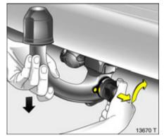
Dismounting the coupling ball bar Open the protective flap and turn the key to position 1 to unlock the coupling ball bar
