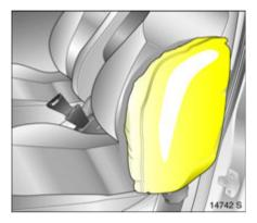
When deployed, the side airbag inflates within milliseconds to form a safety cushion for the driver or front passenger in the respective front door area. This substantially reduces the risk of injury to the upper body and pelvis in the event of a side-on collision.
