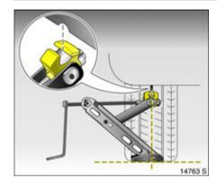
The edge of the jack base must be planted firmly and vertically in line with the contact point.
