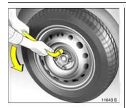
2. Push the wheel bolt wrench \* on as far as possible and slacken the wheel bolts half a turn.
