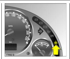
Illuminates while driving: Fault in the system. Driving can be continued. Poor road surface conditions may however still cause vehicle stability to be impaired.
