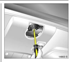
Use a screwdriver \* to push the drive shaft in and turn until the sunroof or slide/tilt roof is closed.
