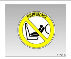
Vehicles with front passenger airbag can be recognised by the word **AIRBAG** above the glove compartment and by the sticker on the instrument panel on the passenger side - see Fig. 11704 A.
