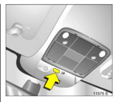
Activation without monitoring of passenger compartment and vehicle tilt Switch on e.g. if animals are to be left in the vehicle.
