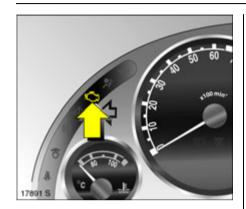
Control indicator ♥ for exhaust Illuminates when the ignition is switched on and during the start attempt. Goes off shortly after the engine starts running.
