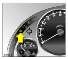
Control indicator for immobilizer & か Control indicator & illuminates briefly when the ignition is switched on.
