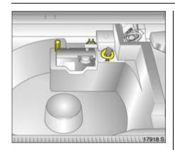
Screw in the towing eye anticlockwise as far as it will go until it stops in a horizontal position.
