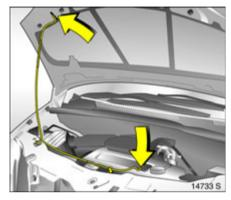
Secure the bonnet support. Before closing the bonnet, press the support into the holder.
