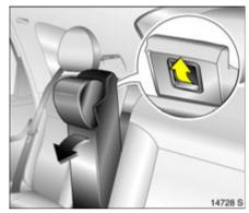
Fold the centre seat forward and lower. House centre seat belt in the holder in the ceiling  $\triangleright$  63.
