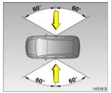
The curtain airbag system will be triggered:
