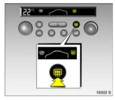
Heating works with the engine running and is switched off automatically after a few minutes.
