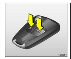
The remote control has a range of approx. 5 metres. This range can be affected by outside influences. Aim the remote control at the vehicle to operate. The hazard warning lamps flash to confirm remote control operation.
