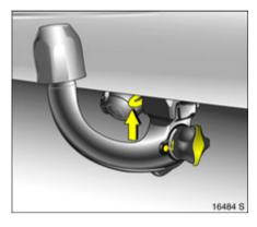
Lock the coupling ball bar in position by turning key to position 2 ▷ 159, Fig. 12416 T. Remove the key and press the protective flap into place.
