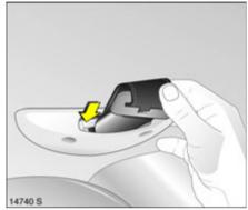
Insert in the seat belt holder in the roof with the lower latch plate pointing forward.
