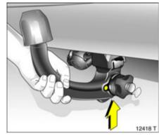
Inserting the coupling ball bar Insert the tensioned coupling ball bar in the housing and push firmly upwards until it audibly engages.
