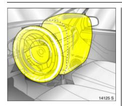
When triggered, the front airbags inflate in milliseconds to form a safety cushion for the driver and front passenger. The forward movement of the front seat occupants is checked, thereby substantially reducing the risk of injury to the upper body and head.
