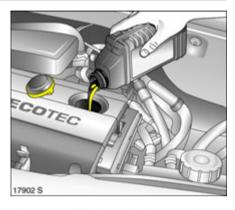
The amount filled must be between the MIN and MAX marks \$\times 230.
