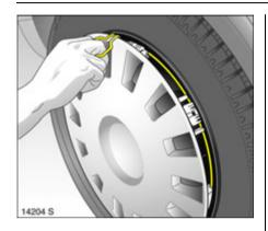
1. Pull off the wheel trim with the hook \*. Vehicle tools \$\times\$ 171.
