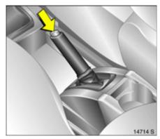
Releasing the hand brake: Raise lever slightly, Press release button, Lower lever fully Hand brake \$\times\$ 153.
