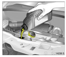
The engine oil level must not exceed the MAX mark on the dipstick.
