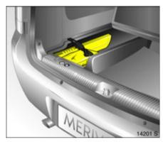
To open, remove the luggage compartment cover **\*** ▷ 55, lift the floor using the handle and raise toward the front.
