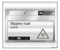
In vehicles with graphical information display \* or colour information display \*, a warning message Slippery road appears on the display as a warning for icy road surfaces. There is no message below -5  $\Box$ C.
