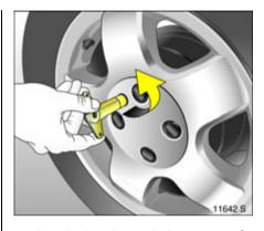
Alloy wheels with anti-theft protection \*: unscrew hubcaps using the wheel nut socket and remove. Vehicle tools \$\sime\$ 171.
