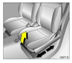
To adjust front seat leg room: Pull handle, slide seat, release handle Seats  $\diamondsuit$  44, Seat position  $\diamondsuit$  45.
