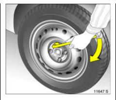
If the wheel bolts have retaining washers \*, they must not be removed.
