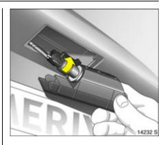
2. Rotate bulb holder to left and disengage.
