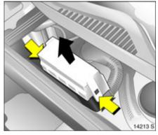
Fuse box in engine compartment The fuse box is at the front left of the engine compartment.
