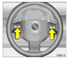
Horn: Press ► Airbag system \* \$\phi\$ 67, Steering wheel remote control \* \$\phi\$ 111.
