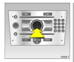
Selection using multifunction button \*: rotate and press multifunction button.
