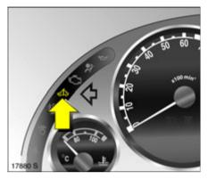
Control indicator & for engine electronics Illuminates for a few seconds after the ignition is switched on.
