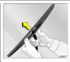
Wiper blade on the rear window  $\divideontimes$ Lift wiper arm. Disengage wiper blade as shown in illustration and remove.
