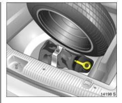
The towing eye is in the tool kit \* in the luggage compartment underneath the spare wheel \*, see Fig. above, or for versions with tyre repair kit \*, in the storage compartment underneath the floor cover, see Fig. 17918 S.
