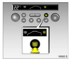
On vehicles with electronic climate control  $\frak{\mbox{\sc m}}$  appears on the climate control display.
