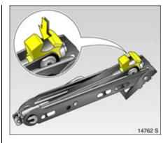
4. Set the jack \* to the required height by turning the lug by hand. Fit the jack arm at the front – or rear – so that the jack claw (arrow in Fig.) grasps the vertical ridge and engages in the recess in the ridge. Ensure that the claw is properly positioned.
