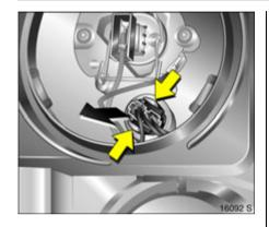
Push side lugs of parking lamp holder together and remove holder from reflector.
