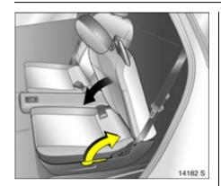
Grasp the backrest, pull the handle at the outboard side of the seat and fold the backrest onto the seat. Release the handle and engage the backrest.
