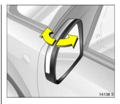
For the safety of pedestrians, the exterior mirrors will swing out of their normal mounting position if they are bumped with sufficient force. Reposition the mirror by applying slight pressure to the mirror housing.
