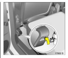
Hook the net straps into slots on the outer seat bracket of the front seats and tighten.
