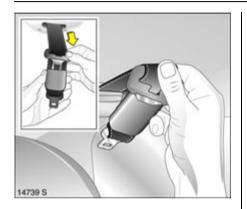
To remove the seat belt, press the button on the left buckle (2). If the centre seat is lowered, press the button on the right buckle (1). The seat belt retracts automatically.
