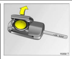
Remote control battery replacement Replace the battery as soon as the range of the remote control begins to shrink.
