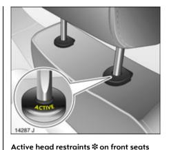
In the event of a rear-end impact, the active head restraints automatically tilt slightly forward. The head is more effectively supported by the head restraint
