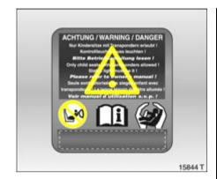
Vehicles with seat occupancy recognition can be identified by the sticker on the front passenger seat or on the side of the instrument panel.
