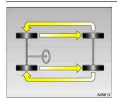
If wear in the front is greater than that in the rear, move the rear wheels to the front axle and vice versa.
