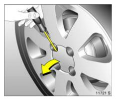
Alloy wheels **∜**: Prise off the hub cap by inserting a screwdriver \* in the recess at the side of the hub cap. Protect the rim by placing a soft cloth between the screwdriver and the alloy wheel.
