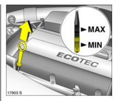
Pull out the dipstick, wipe it clean, insert it to the stop on the handle, pull out and read the engine oil level.
