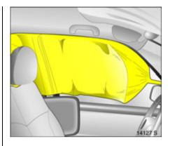
When the curtain airbag is triggered it inflates within milliseconds and provides a safety barrier in the head area on the respective side of the vehicle. This reduces the risk of injury to the head considerably in case of a side impact.
