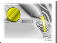
Top up with the same brand of engine oil that was used during the previous engine oil change, following the instructions in the chapter "Service, Maintenance" on page 165.
