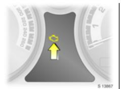
Control indicator (a) for exhaust Illuminates when the ignition is switched on and during the start attempt. Goes out shortly after the engine starts running.
