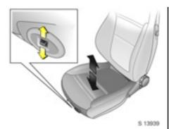
Adjust driver seat height Press and hold switch up or down until desired position is reached.
