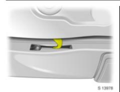
Ensure the retaining hook is correctly aligned within its aperture before attempting to engage the locking lever.
