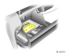
The service parts identification label is located in the glove compartment.
