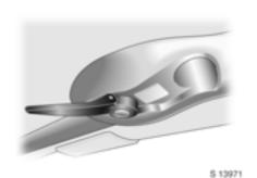
To avoid damaging the soft top or the roof mechanism, the lever must remain in the open position during the lowering procedure.
