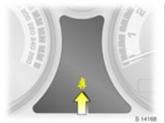
Driver's seat belt warning device & Control indicator & illuminates in the instrument panel for approx. 20 seconds when the ignition is switched on, or until driver's seat belt is fastened. Flashes for a further 60 seconds if seat belt remains unfastened.
