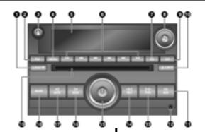
0 1...6 Preset buttons 1 to 6 Select options in corresponding display panel labels Radio: View and save favourite stations 0 ΕQ Select preset equalisation settings: Press 0 Adjust sound settings: Press and turn CD: Select track; turn Radio: Select station; turn 0 CAT Change category CD: Toggle between CD audio and MP3 files
