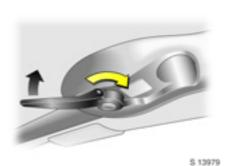
Engage the locking lever by rotating it clockwise and pushing it up. The retaining hook will hook into position.
