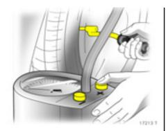
After having checked the tyre pressures, tighten the valve caps.
