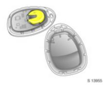
Remove used battery, taking care to avoid touching any of the circuitry.
