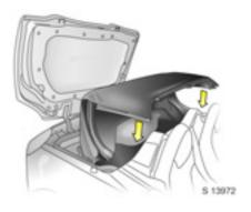
From the side of the vehicle, pull the soft top away from the windscreen frame and fold it down into the luggage compartment.
