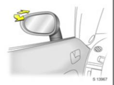
For the safety of pedestrians, the exterior mirrors will swing out of their normal mounting position if they are bumped with sufficient force. Reposition the mirror by applying slight pressure to the mirror housing.
