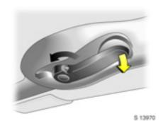
Release the locking lever located in the centre of the header rail by pulling it down and rotating it anti-clockwise. The retaining hook will unhook.
