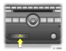
Control indicator  $\Re_2$  illuminates continuously as soon as the system has detected that the passenger's seat is occupied and the passenger is correctly seated. When a passenger occupies the passenger's seat, the airbag for the passenger's seat is activated and may inflate in the event of an accident.
