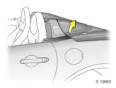
With soft top in raised position, the buttresses are unlatched automatically before the luggage compartment is opened. Soft top - see page 31.
