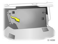
To open, pull cover from the left-hand side to detach from Velcro pads and remove cover.
