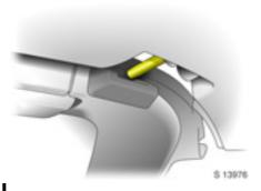
Fully raise the soft top ensuring the alignment pins locate correctly in both sides of the windscreen frame and on each side of the body adjacent to the seat backrests.
