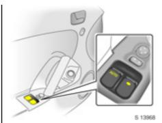
The driver's and passenger's window are operated via the switches located in the driver's door handle.
