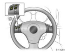
Accelerate to the desired speed, press the - SET button and release it: the current speed is stored and maintained.
