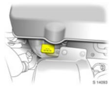
The negative jump start terminal is identified by a "GND (-)" sign on a ground bracket, located below the engine beauty cover.
