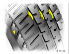
The legally permissible minimum tread depth (1.6 mm) has been reached when the tread has worn down as far as one of the wear indicators (TWI<sup>1</sup>). A number of wear indicators are spaced at equal intervals around the tyre within the tread. Their position is indicated by markings on the tyre sidewall.
