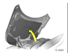
To open completely, lift bonnet upwards from the edge nearest the windscreen. Air pressurised support rods will hold the bonnet open.
