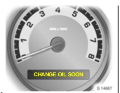
The engine oil life monitor lets you know when to change the engine oil. Based on driving conditions, the time or kilometre/mileage interval at which an engine oil change will be indicated can vary considerably.
