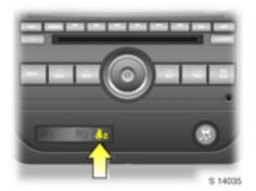
Passenger's seat belt warning device \$\frac{4}{2}\$ Control indicator \$\frac{4}{2}\$ illuminates in the centre console after approx. 20 seconds when the ignition is switched on, if passenger's seat belt is unfastened and the seat occupancy recognition system detects that the passenger's seat is occupied. Stays illuminated for a further 20 seconds then flashes for approx. 60 seconds if seat belt remains unfastened.
