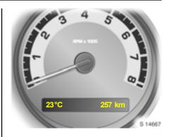
Outside temperature and odometer Displays outside temperature and record of total kilometres/miles driven (odometer) when the ignition is on.
