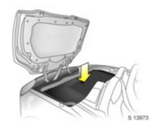
To allow the luggage compartment lid to close correctly, ensure the soft top is properly stowed by applying a firm, even push in the centre of the soft top.
