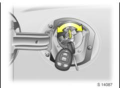
Fuel filler neck at left rear side of vehicle. Open the tank flap.
