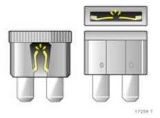
A blown fuse can be recognised by its melted wire. Do not install a new fuse until the cause of the fault has been remedied. Different types of fuse are used.
