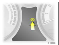
Control indicator (1) for brake system Illuminates when the ignition is switched on if the hand brake is applied or if the brake/clutch fluid level is too low.
