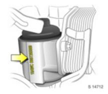
Engine identification: etched into the engine oil filter housing on the cylinder block.
