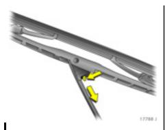
To replace wiper bla de, lift wiper a m aw ay from windscreen. Move release lever a nd detach wiper blade.
