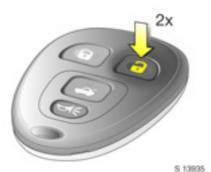
To unlock and open the doors: Press button don remote control to unlock driver's door, pull door handle
