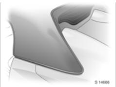
Press the buttresses into the corresponding apertures on either side of the vehicle with a swift, firm motion, ensuring they are latched correctly into the top of the lugg age compartment lid.
