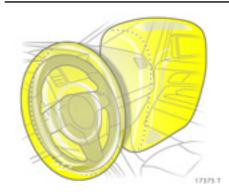
When triggered, the airbags inflate in milliseconds to form a safety cushion for the driver and passenger. The forward movement of the seat occupants is checked, thereby substantially reducing the risk of injury to the upper body and head.
