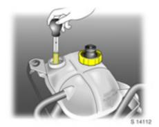
Antifreeze and corrosion protection Before the start of the cold weather season, have the coolant checked for correct concentration.
