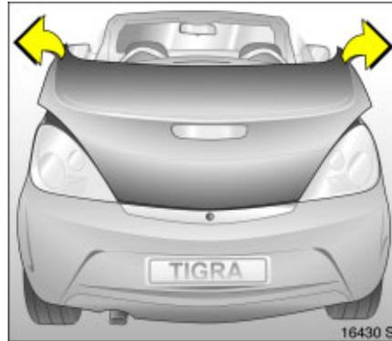
13. With two people working simultaneously on the right and left, open the boot lid rearward to its end position. Do not twist or tilt the boot lid when doing so.
