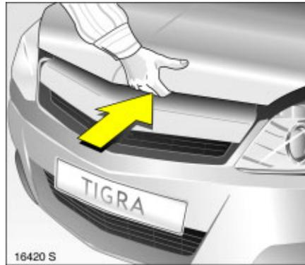
Pull the safety catch upwards and open the bonnet.
