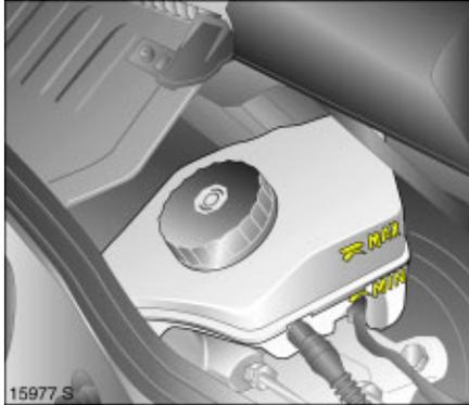
The brake fluid must be between the **MIN** and the **MAX** marks.
