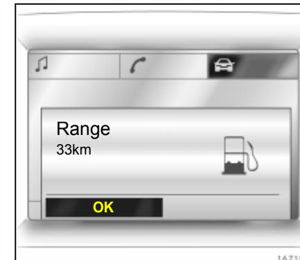
If the fuel in the tank will allow less than 50 km of travel, the message **Range** appears in the display.
