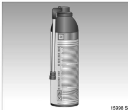
The tyre repair aerosol allows for temporary use of the tyre; it merely allows for continued travel until the tyre can be changed.
