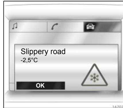
In vehicles with graphical information display ❄️, the warning message **Slippery road** is shown in the display as a warning for icy road surfaces. No message is displayed at temperatures below -5 °C.
