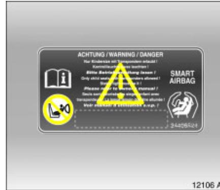
Use of a child restraint system \* on the front passenger seat of a vehicle with seat occupancy recognition \*
