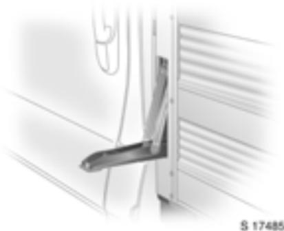
Pull the lever down until it contacts the body and lower the sideboard carefully.
