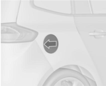
The fuel filler flap can only be opened if the vehicle is unlocked. Release the fuel filler flap by pushing the flap.
