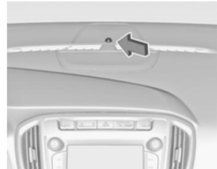
Status LED is integrated into the sensor on top of the instrument panel.
