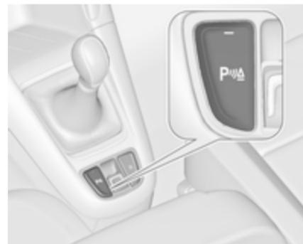
Manual deactivation is also possible by pressing the parking assist button **P**▲.
