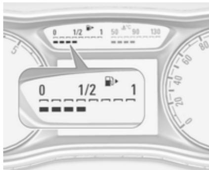
Displays the fuel level or gas content (LPG or CNG) in the tank depending on the operation mode.
