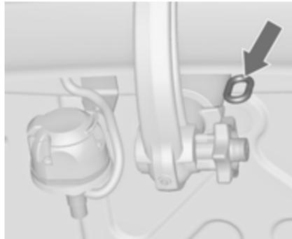
Attach breakaway stopping cable to eye.
