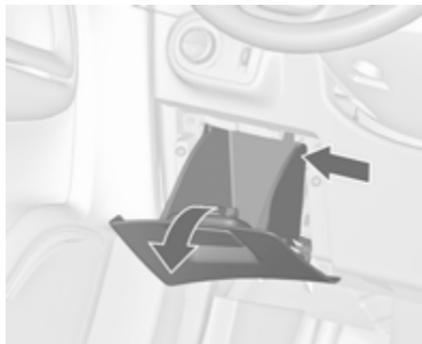
In left-hand drive vehicles, the fuse box is behind the storage compartment in the instrument panel. Open the compartment and push it to the left to unlock. Fold the compartment down and remove it.
