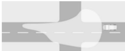
Activated automatically at a speed up to approx. 55 km/h. In situations with exterior ambient light both cornering lights are switched on with reduced intensity. The light is wide and symmetrical.
