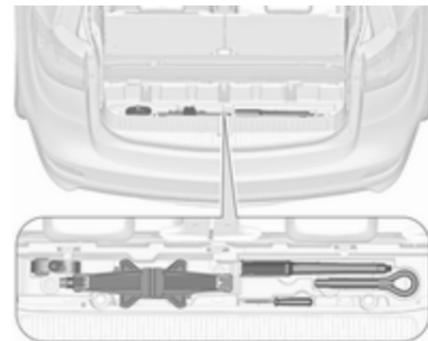
Some tools, the towing eye and (only on vehicles with spare wheel) the vehicle jacking equipment are placed in the rear storage in the load compartment floor.
