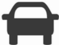
The green illuminated vehicle ahead control indicator
