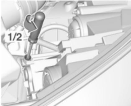
There is a white adjuster element on the rear of each headlight housing.
