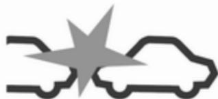
When the distance to a preceding moving vehicle gets too small or when approaching another vehicle too rapidly and a collision is imminent the collision alert symbol pops-up in the Driver Information Centre and a warning chime sounds. Depress the brake pedal, if it is required by the situation.
