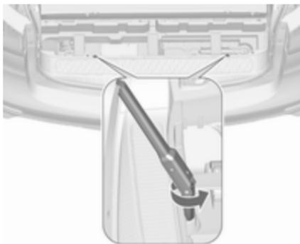
3. Fit the wheel wrench on one hexagon bolt and turn it anticlockwise until a resistance is noticeable.
