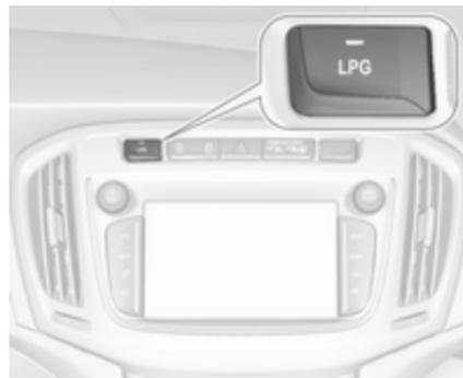
Press **LPG** to switch between petrol and liquid gas operation. The LED
