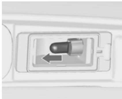
2. Remove the bulb from the socket by pulling.
