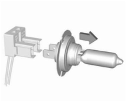
3. Remove the bulb from the plug connector by pulling.
