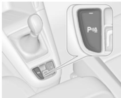
An illuminated LED in the parking assist button **P**▲ indicates that the system is ready to operate.
