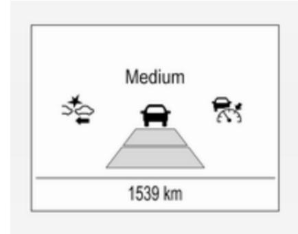
Note that the alert timing sensitivity setting is shared with the following distance setting of the adaptive cruise control. So changing the alert timing sensitivity changes the adaptive cruise control following distance setting.
