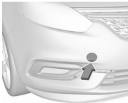
Disengage cap at bottom and remove downwards.
