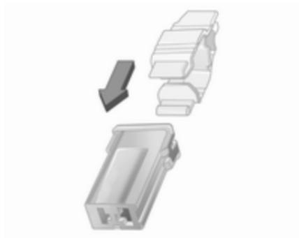
Place the fuse extractor on the various types of fuse from the top or side, and withdraw fuse.
