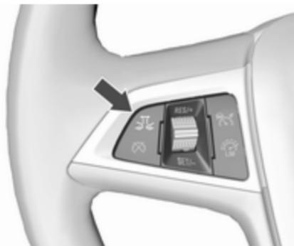
Press **SET/-**, the current setting is shown in the Driver Information Centre. Press **SET/-** again to change the following distance. The setting is also displayed in the Driver Information Centre.
