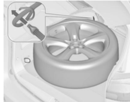
2. Place the loop end of the strap through the front lashing eye on the left side.
