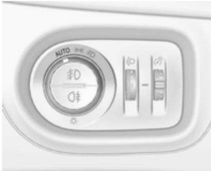
When the automatic light control function is switched on and the engine is running, the system switches between daytime running lights and headlights automatically depending on the external lighting conditions and information given by the rain sensor system.
