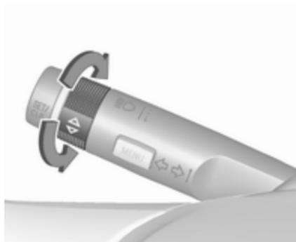
Turn the adjuster wheel to select a submenu of the main menu or to set a numeric value.
