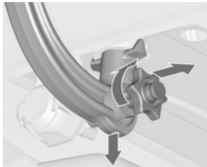
Open the protective flap and turn the key to position
