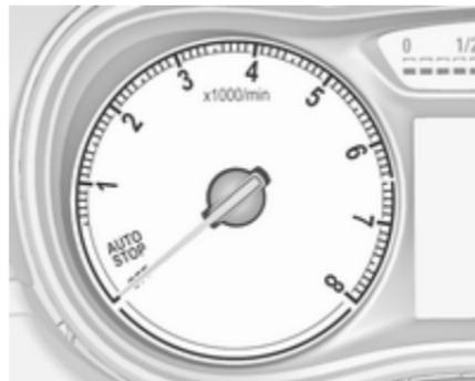
Displays the engine speed.
