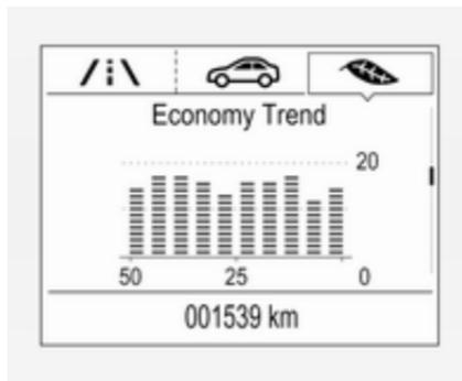
Displays the average consumption development over a distance of 50 km. Filled segments display the consumption in 5 km steps and shows the effect of topography or driving behaviour on fuel consumption.
