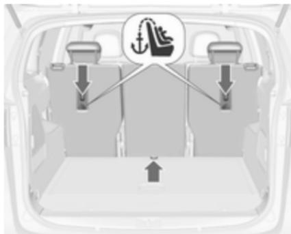
In addition to the ISOFIX mounting brackets, fasten the Top-tether strap to the Top-tether fastening eyes. The strap must run between the two guide rods of the head restraint.
