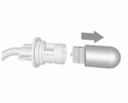
3. Pull bulb from bulb holder and replace it.
