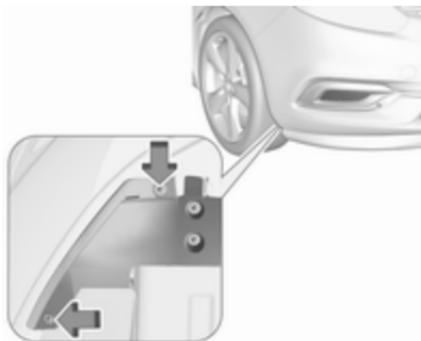
1. Remove the outer screws of the cover, as shown in the illustration.
