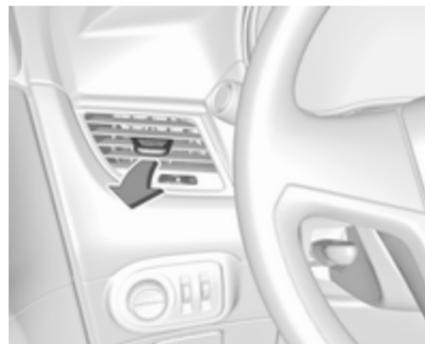
To close the vent, turn the adjuster wheel to **O**.
