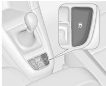
TC can be switched off when spinning of drive wheels is required: press
