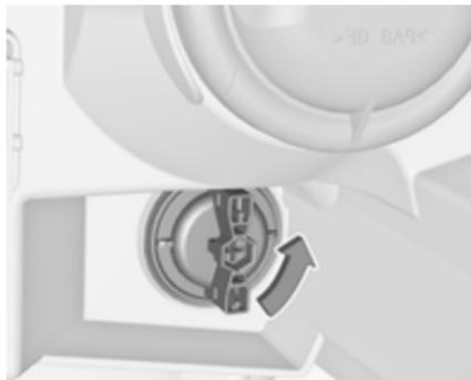
1. Rotate bulb socket anticlockwise to disengage. Withdraw the bulb socket from the reflector housing.
