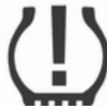
A detected low tyre pressure condition is indicated by control indicator 115.
