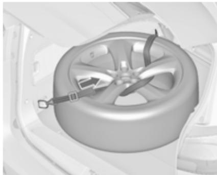
4. Insert the strap through the spokes of the wheel as shown in the illustration.
