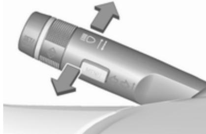
Push lever to switch from low to high beam.
