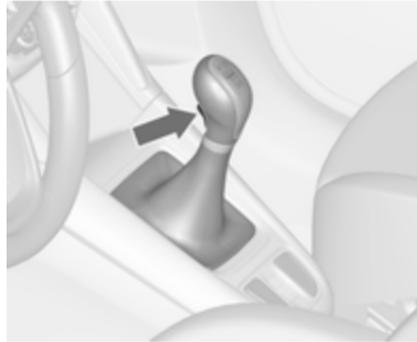
To engage reverse, depress the clutch pedal and then press the release button on the selector lever and engage the gear.
