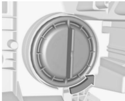
1. Rotate cap anticlockwise and remove it.
