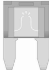
Depending on the type of fuse, a blown fuse can be recognized by its melted wire. Do not replace the fuse until the cause of the fault has been remedied.
