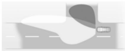
On tight bends or when turning off, depending on the steering angle or the indicator light signal, an additional left or right reflector is switched on which illuminates the road in the direction of travel. It is activated up to a speed of 70 km/h.
