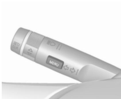
Press **MENU** to switch between the menus or to return from a submenu to the next higher menu level.
