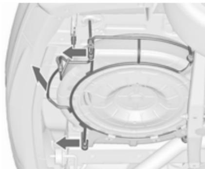
5. Lift the spare wheel holder and unhook both catches.
