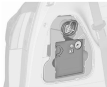
If equipped with tyre repair kit, remove the complete box.
