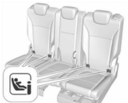
Fasten vehicle-approved ISOFIX child restraint systems to the ISOFIX mounting brackets. Specific vehicle ISOFIX child restraint system positions are marked in the ISOFIX table ⇨ 63.
