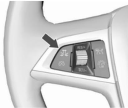
Press ; the current setting is shown in the Driver Information Centre. Press again to change the alert sensitivity. The setting is also displayed in the top line of the Driver Information Centre.
