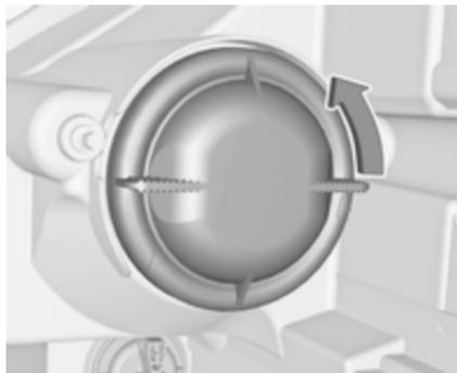
1. Rotate cap anticlockwise and remove it.
