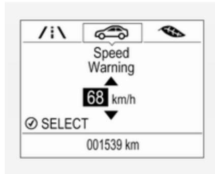
The speed warning function alerts the driver when a set speed is exceeded.
