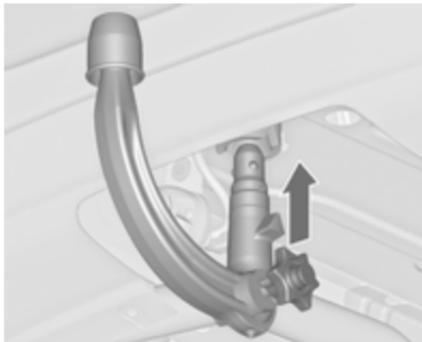
Insert the tensioned coupling ball bar in the opening and push firmly upwards until it audibly engages.
