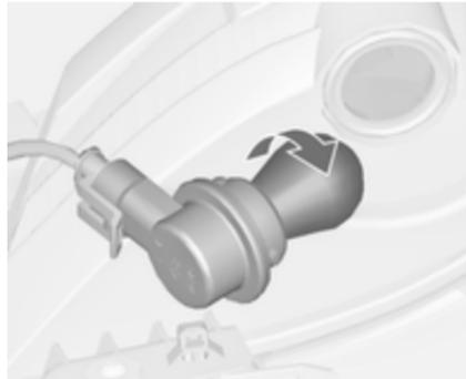
2. Remove the bulb from the socket by turning anticlockwise.
