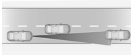
If another vehicle enters your driving path, adaptive cruise control will first consider the vehicle when it is completely in your path. Be ready to take action and depress the brake pedal, if you need to brake more quickly.
