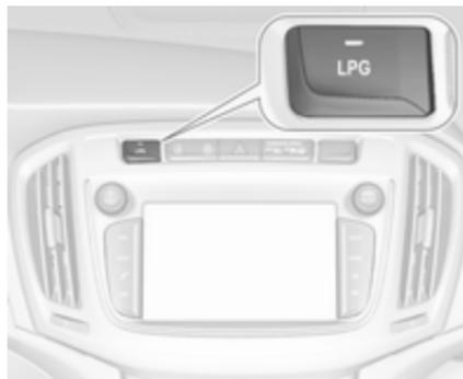
Pressing **LPG** switches between petrol and liquid gas operation as soon as the required parameters (coolant temperature, gas
