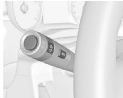
Select Vehicle Information Menu
