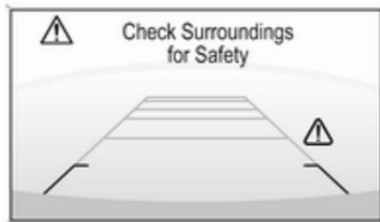
Due to the high position of the camera, the rear bumper can be seen on the display as a guide to position. The area displayed by the camera is limited. The distance of the image that appears on the display differs from the actual distance.
