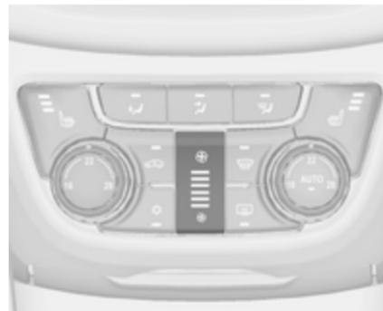
Press the lower button to decrease or upper button to increase fan speed. The fan speed is indicated by the number of segments in the display.
