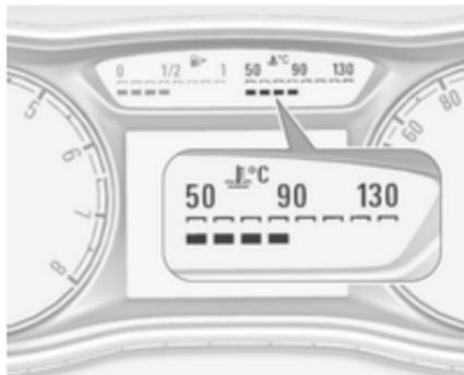
Number of LEDs displayed shows the coolant temperature.
