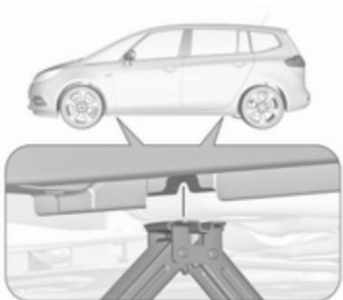
4. Ensure the jack is correctly positioned under the relevant vehicle jacking point.
