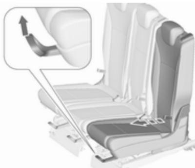
When using ISOFIX fastened child restraint systems on the second seat row, we recommend to adjust the accordant outer seat in third notch from rear end position, regarding to base seats. Lounge seat, if equipped, must be in normal position ⇨ 44.
