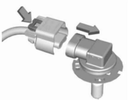
3. Disengage the bulb socket from the plug connector by pressing the retaining lug.
