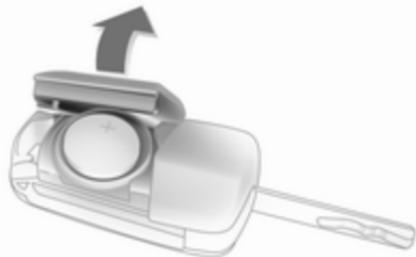
Extend the key and open the unit. Replace the battery (battery type CR 2032), paying attention to the installation position. Close the unit and synchronise.
