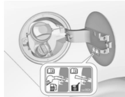
The misfuel inhibitor ensures that the flap of the fuel filler neck can only be opened by using a nozzle for diesel fuel or a funnel for emergency refilling.
