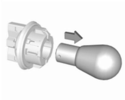
2. Remove the bulb from the socket by turning anticlockwise and pulling.
