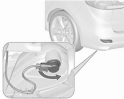
1. Turn the bulb socket anticlockwise and remove it from the reflector.
