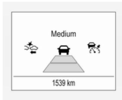
The selected following distance is indicated by filled distance bars on the adaptive cruise control page.
