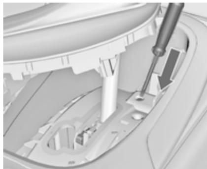
3. Push down the release lever and move the selector lever out of **P** or **N**. If these positions are engaged again, the selector lever will be locked in position again. Have the cause of the power supply interruption remedied by a workshop.
