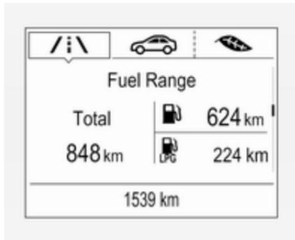
Display of the approximate total fuel range and for each fuel tank (LPG or CNG and petrol). A low fuel level in either tank is indicated by **Low** in the respective section.
