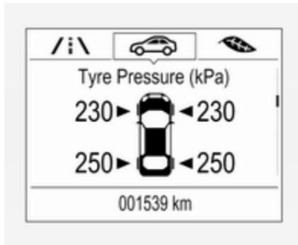
6. Press **SET/CLR** to begin the sensor matching process. A message requesting acceptance of the process should be displayed.
