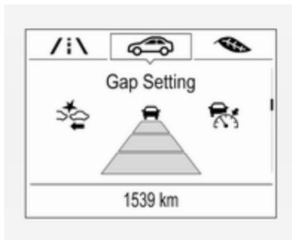
If Adaptive cruise control is active, this page shows the alert sensitivity setting instead of following distance setting. ↗ 176.
