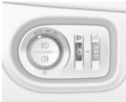
To adapt headlight range to the vehicle load to prevent dazzling: turn thumb wheel
