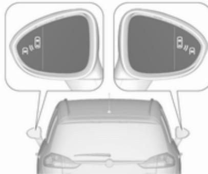
Side blind spot alert is active from speeds of 10 km/h up to 140 km/h. Driving faster than 140 km/h deactivates the system, indicated by low lighting warning symbols
