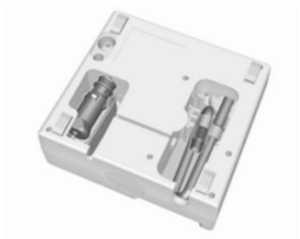
3. Remove the electrical connection cable and air hose from the stowage compartments on the underside of the compressor.
