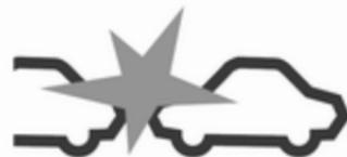
If a vehicle directly ahead is approached too quickly, a warning chime and alert in the Driver Information Centre is provided.
