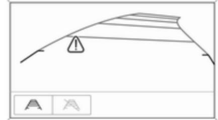
**7" R 4.0 IntelliLink** Activation or deactivation of the visual guiding lines and the warning symbols can be changed via touch buttons in the lower zone of the display.
