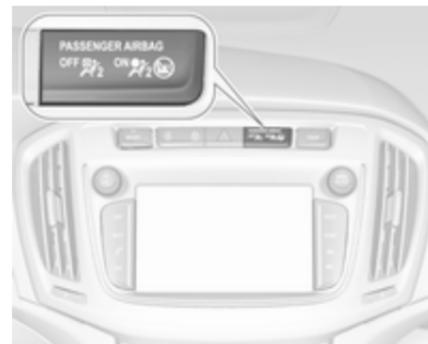
If the control indicator **ON**
