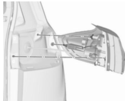
3. Carefully withdraw the light assembly from the retaining pins and remove.
