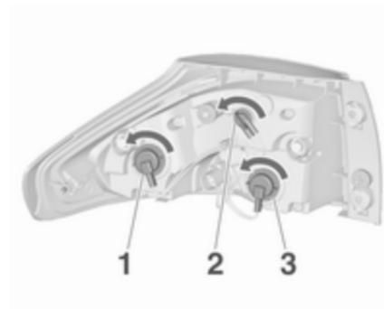
5. Remove and replace the bulb by turning the bulb socket.
