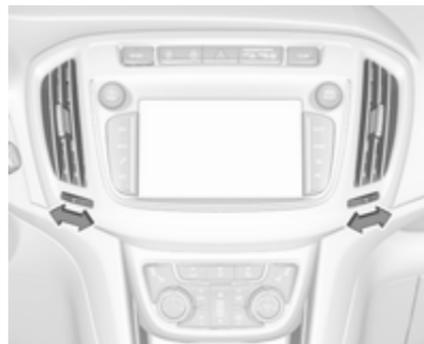
To open the vent, turn the adjuster wheel to **I**. Adjust the air amount at the vent outlet by turning the adjuster wheel.
