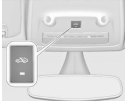
Switch off the monitoring of passenger compartment and vehicle inclination when animals are being left in the vehicle, because of high volume ultrasonic signals or
