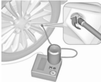
6. Unscrew valve cap from defective tyre.
