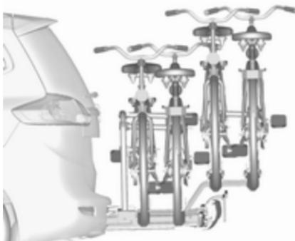
The rear carrier system (Flex-Fix system) allows two bicycles to be attached to an extendable carrier integrated into the vehicle floor. It is possible to attach two further bicycles on an adapter. The transportation of other objects is not permitted.
