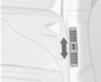
Air vents for rear passenger are left and right side behind the front seats.
