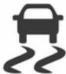
ESC is operational after each engine start as soon as the control indicator
