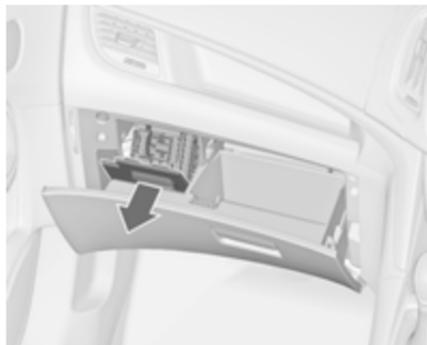
In right-hand drive vehicles, the fuse box is located behind a cover in the glovebox. Open the glovebox, then open the cover and fold it down.
