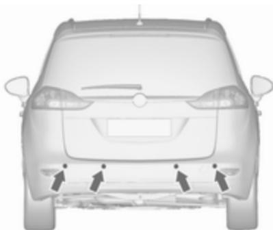
The system has four ultrasonic parking sensors each in the rear and front bumper.
