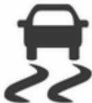
TC is operational after each engine start as soon as the control indicator
