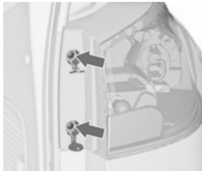
2. Remove the screws, marked by the arrows.
