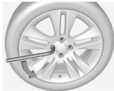
1.1. Insert extractor in the open slot of the centre cap and remove the cap from the wheel. Vehicle tools ⇨ 186.
