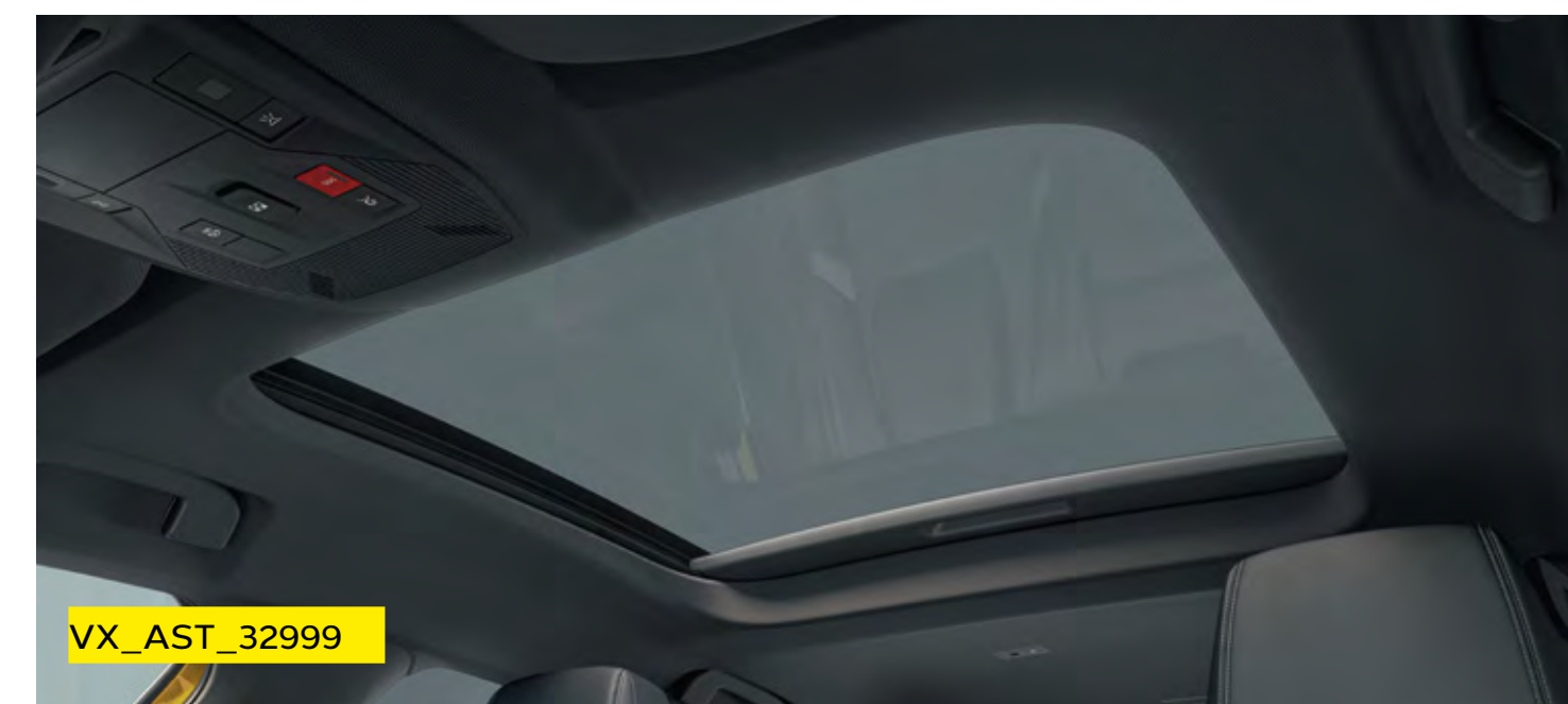
Electrically operated slide/tilt glass sunroof with blind.
