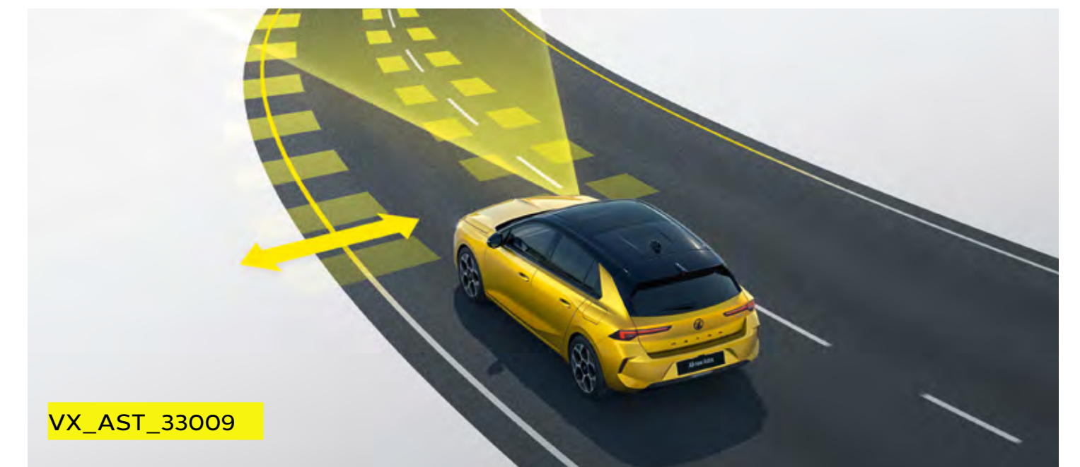
Lane departure warning with lane keep assist.
