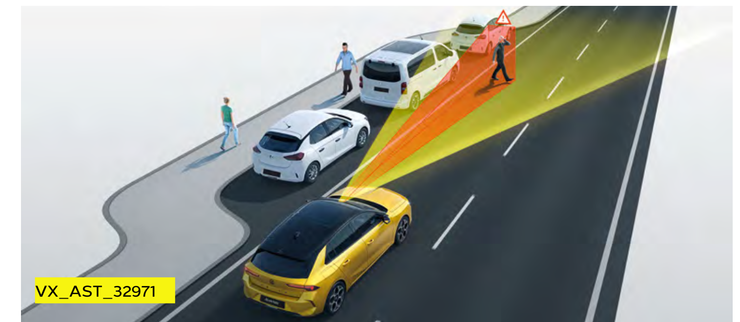
Automatic emergency braking with pedestrian detection.
