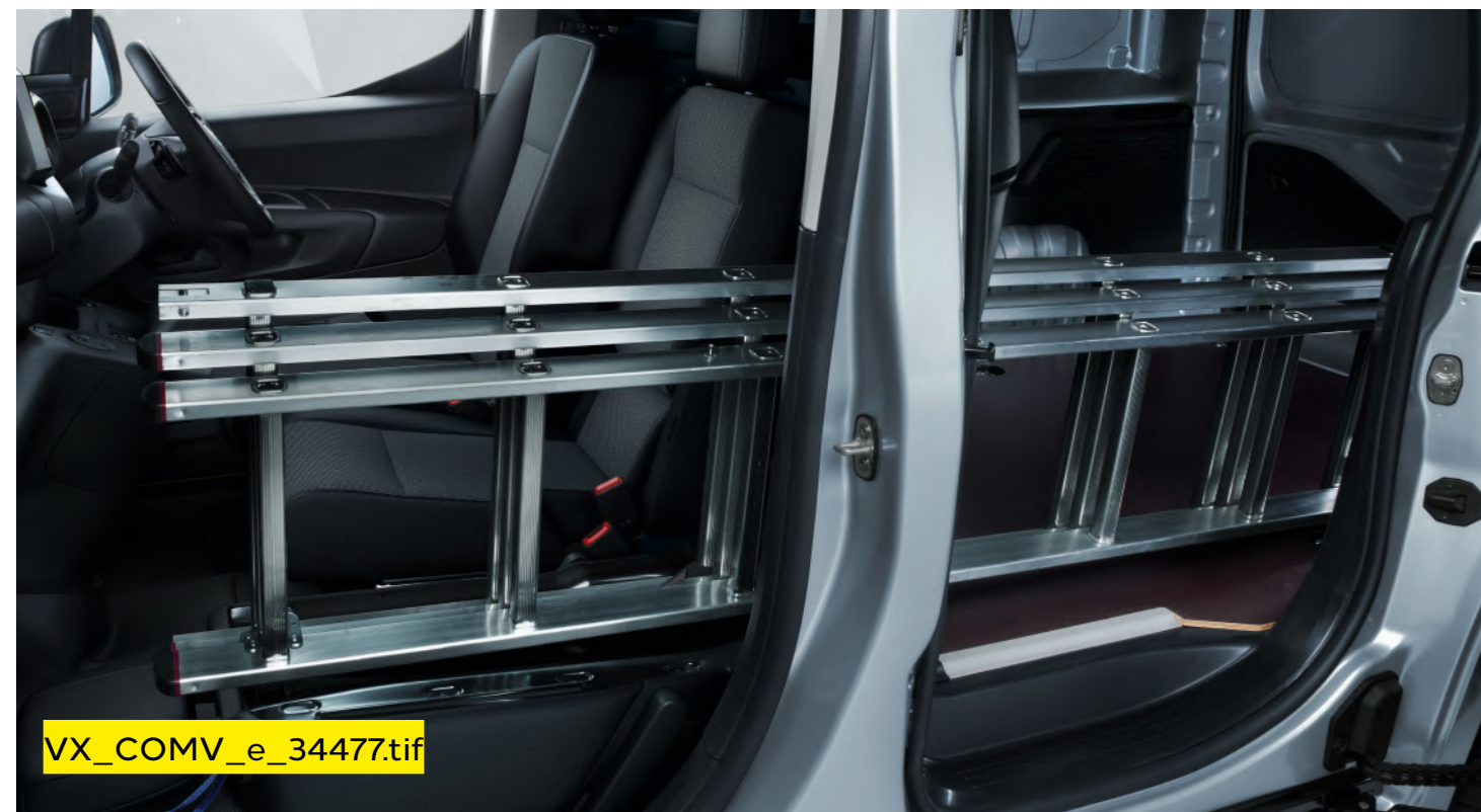
Load-through hatch within bulkhead.
