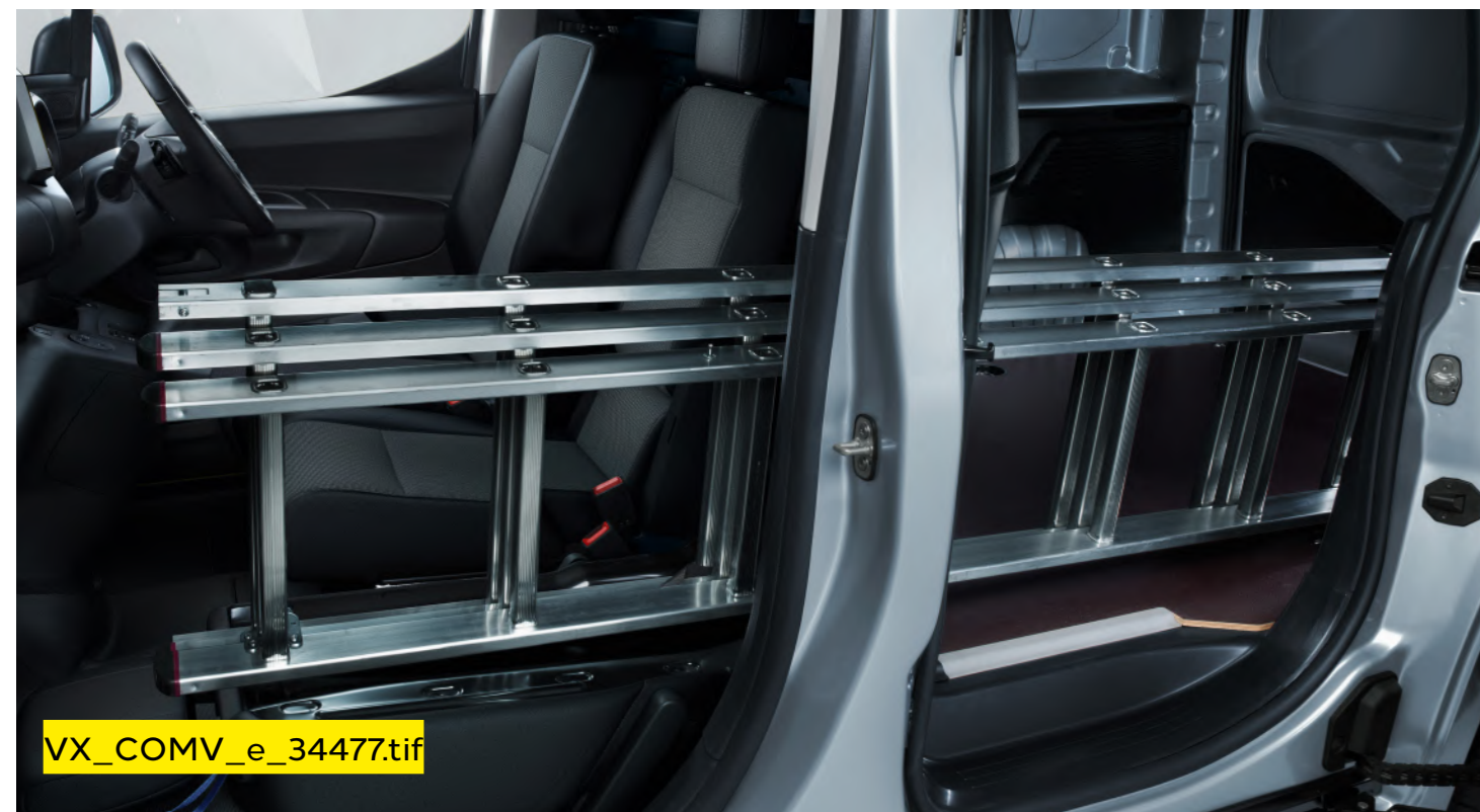
Load-through hatch within bulkhead.
