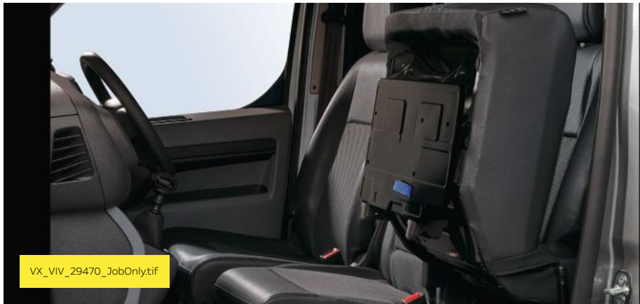
Load-through hatch within bulkhead
