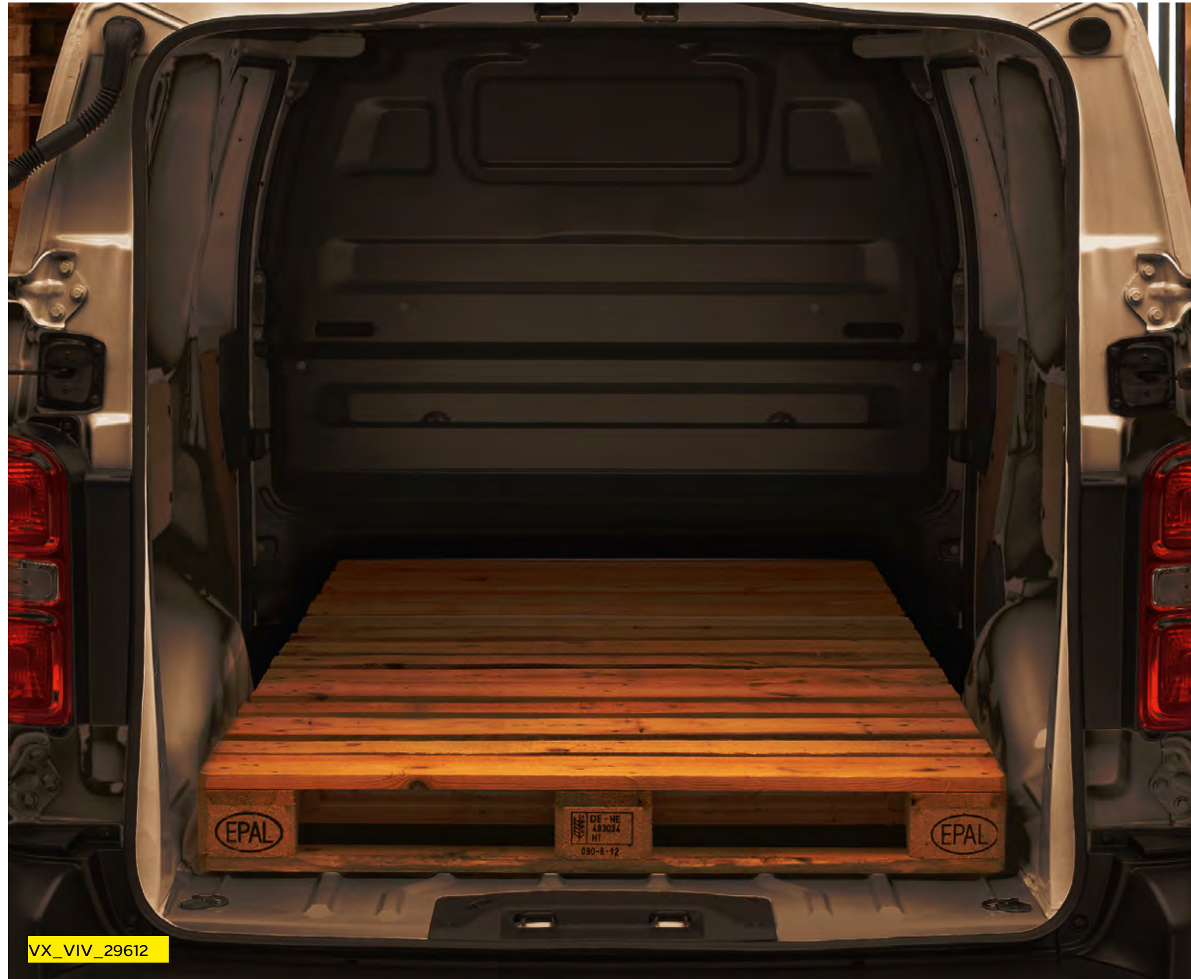
Full-height steel bulkhead.
