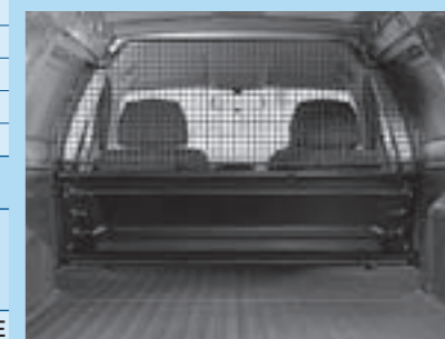
Upper load restraint mesh.
