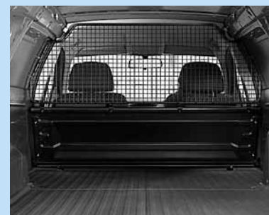
Upper load restraint mesh.
