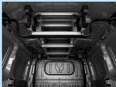
Internal ladder storage bars.
