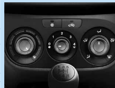
Air conditioning and air recirculation.
