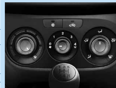
Air conditioning and air recirculation.
