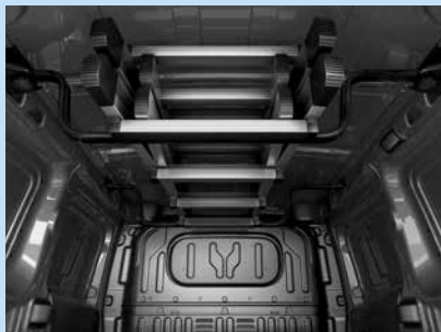
Internal ladder storage bars.
