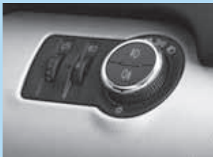
Automatic lighting control.
