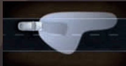
Adverse weather light (up to 45mph). Wiper or rain sensor activated for better vision in bad weather conditions.
