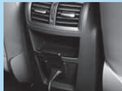
230-volt rear power outlet.
