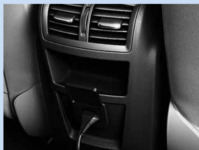
230-volt rear power outlet.
