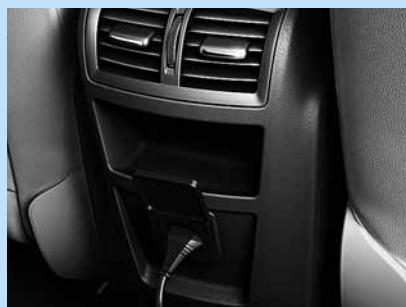
230-volt rear power outlet.
