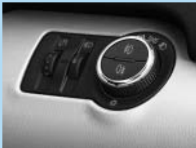
Automatic lighting control.
