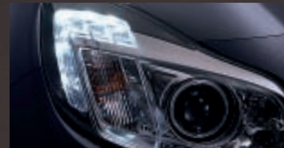
LED Daytime running light. Increases your visibility to other road users without increasing fuel consumption (unlike low beam).
