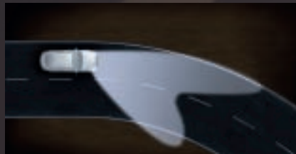
Dynamic curve light (any speed). Activated by steering angle and speed, the headlights swivel up to 15 degrees into the curve.
