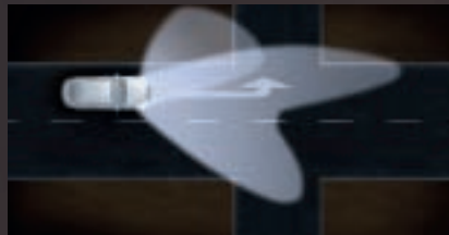
Static cornering light (up to 25mph, also when reversing). Throws light 90 degrees left or right for enhanced lateral vision.
