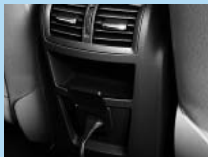
230-volt rear power outlet.
