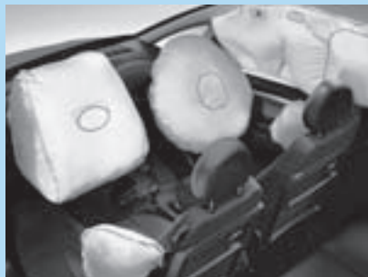
Front seat side-impact and full-size curtain airbags are part of the Protection Pack.
