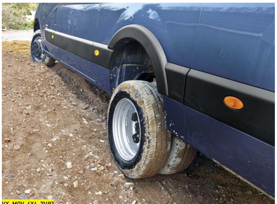
As well as the standard AWD driving mode there is also a low-range mode when more difficult driving conditions prevail such as pulling away under load in tricky off-road conditions. Although the AWD system can also be deployed when driving on harsh road conditions, long term on-road driving with the AWD system engaged is not recommended due to the standard fitment of the lengthwise locking rear differential, transfer case and front axle.
