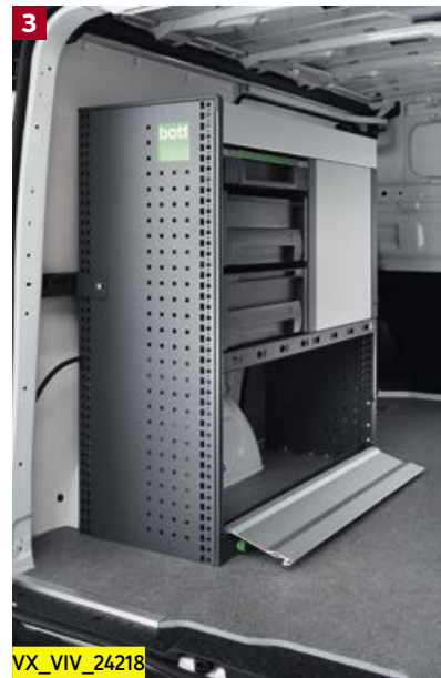
2-3-4. Vivaro L1 H1 featuring fixed shelves with dividers, cupboards, drawers and aluminium drop front.
