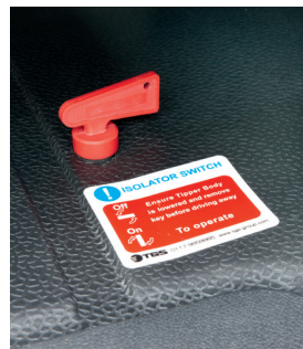
Isolator switch for improved safety.
