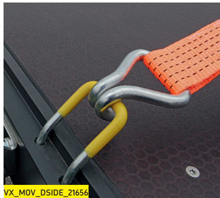
Recessed, wash down lashing eyes.
