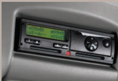
Digital tachograph Computes driving and rest time, enabling fleet management data to be analysed.
