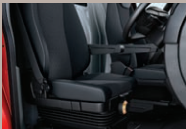
Air-suspended driver's seat Ideal for rough terrain and includes variable suspension sensitivity settings.
