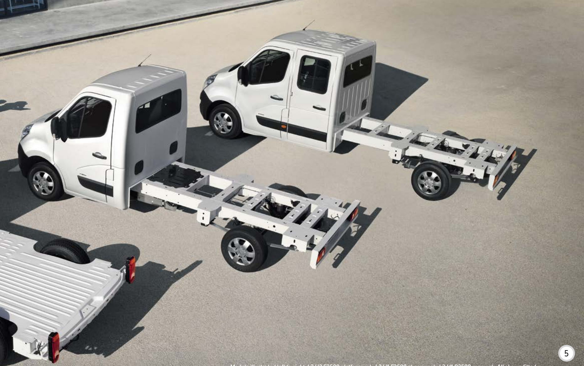
Models illustrated left to right: L2 H2 F3500 platform cab, L2 H1 F3500 chassis cab, L3 H1 R3500 crew cab. All shown fitted with full-size wheel trims, optional at extra cost. Platform cab also features Convenience Pack, optional at extra cost.
