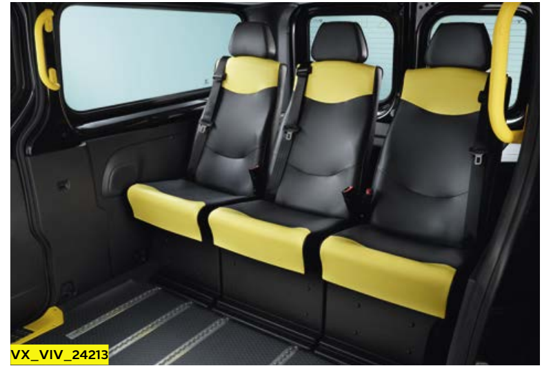
The three rear seats are mounted on quick-release tracking.
