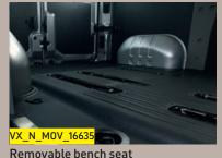
The rear bench seats include floormounted fixing rails so they can be removed without the need for special tools, freeing up additional load area space quickly and easily if required (9-seat model illustrated).
