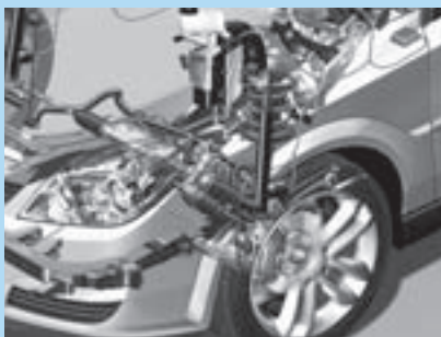
Lightweight MacPherson strut front suspension.
