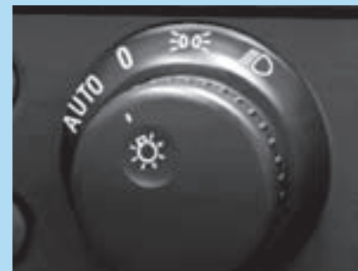
Automatic Lighting Control (ALC)
