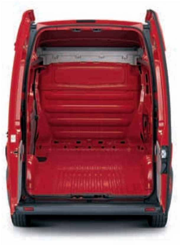
Long wheelbase high roof model illustrated features optional full-height steel bulkhead. A resin-coated wooden load floor covering can also be specified as an option at extra cost if required.
