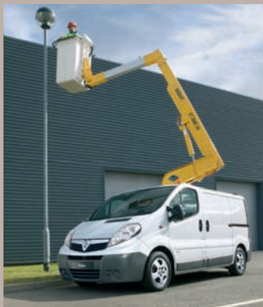
Access platform vans Specifically designed for use without stabilisers.
