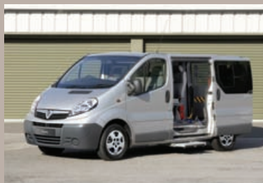
Wheelchair-accessible vehicles Feature two sliding side-access doors and a manually folding rear-access ramp.
