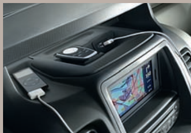
Optional USB facility Allows you to view iPod™ functionality via the audio display.
