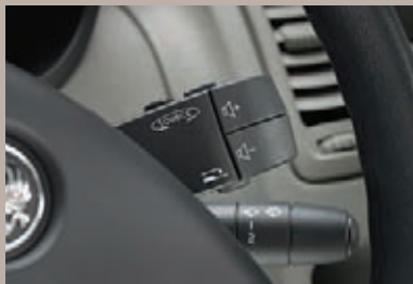
Steering column audio controls. Standard on all Vivaro models, enabling you to operate audio functions.
