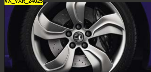
Standard 19-inch five-spoke alloy wheels with 245/40 R 19 ultra-low profile tyres.
