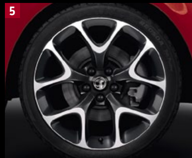
5 18-inch 5 Y-spoke forged bi-colour alloy wheels with 225/35 R 18 ultra-low profile tyres, optional at extra cost
