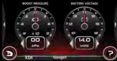
**Gauges.** Select your gauges for real-time information such as Power, Torque, Manifold Pressure, Fuel, Elevation, or Air Temp. (intake or external).
