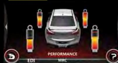
**MRC performance data.** Monitor the performance of the magnetic ride control system in real time (VXR8 GTS models only).
