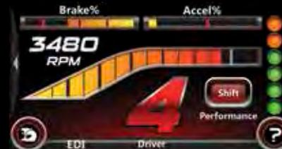
**Driver.** Driver screen keeps you close to key inputs such as RPM, accelerator and brake pedal positions, and gear position.
