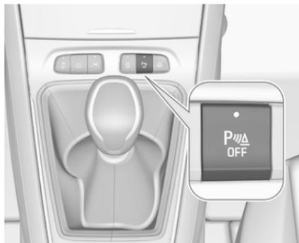
The system is ready to operate when the LED in the parking assist button **P OFF** is not illuminated.
