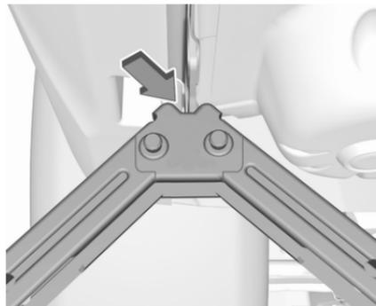
Ensure that the edge of the body fits into the notch of the jack.
