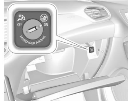
The front passenger airbag system can be deactivated via a key-operated switch in the glovebox.
