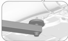
Rear arm position of the lifting platform centrally under the relevant vehicle jacking point.
