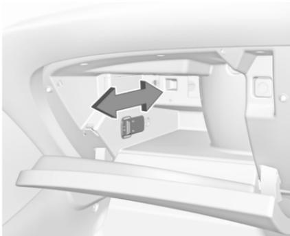
Move the slider back or forth in order to enable or disable glovebox cooling.
