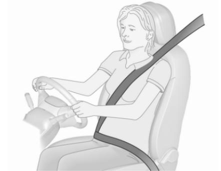
The seat belts are locked during heavy acceleration or deceleration of the vehicle, holding the occupants in the seat position. Therefore the risk of injury is considerably reduced.
