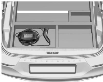
3. Open the tailgate. Lift the rear floor storage cover and remove the charging cable.
