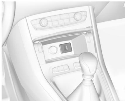
A USB port is located behind the storage cover. Press cover to open.
