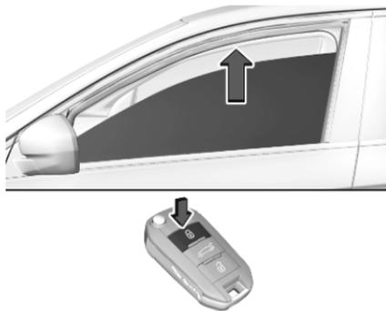
Press and hold
