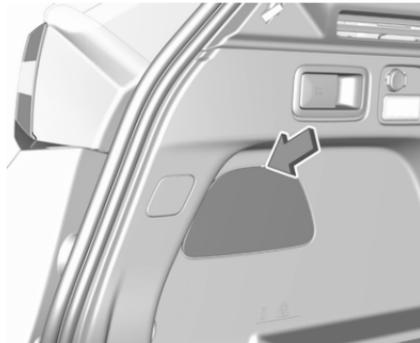
1. Open the tailgate then unclip the access cover on the relevant side.
