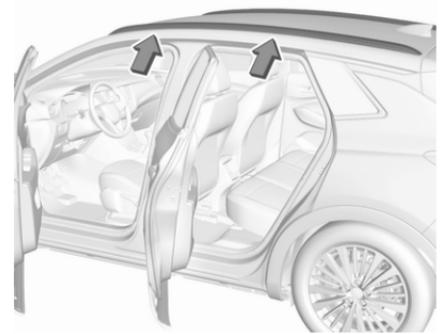
Fasten the roof rack in the roof railing above the mounting points located in each door frame of the vehicle body.
