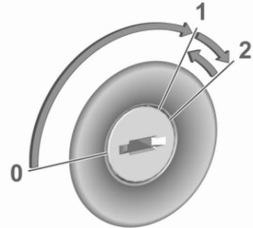
Turn key to position 1 to release the steering wheel lock.
