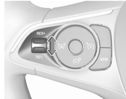
Accelerate to the desired speed and move thumb wheel once briefly to **SET/-**. The current speed is stored as maximum speed.
