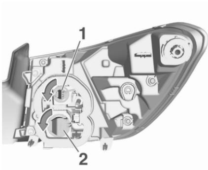
7. Detach the bulb from the bulb socket and replace the bulb.
