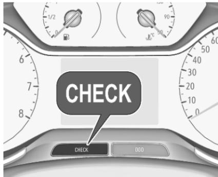
To retrieve the status of the service information at any time press button **CHECK**. The service information is displayed for a few seconds.
