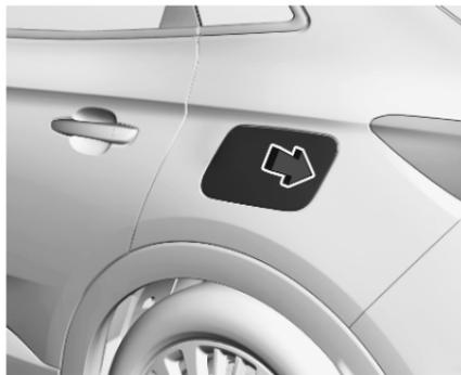
2. Push the rearward edge of the charging port flap in and release to open the flap.
