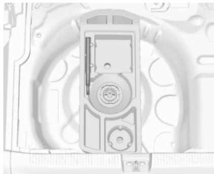
The towing eye and the chocks are located in a box below the floor cover in the load compartment.
