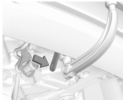
Attach breakaway stopping cable to eye.
