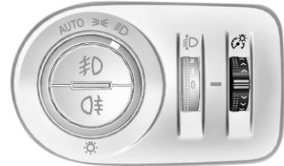
Brightness of the following lights can be adjusted when the exterior lights are on:
