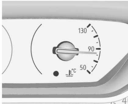
Displays the coolant temperature.
