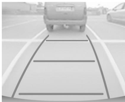
The area behind the vehicle is displayed in the screen. The vertical lines represent the width of the
