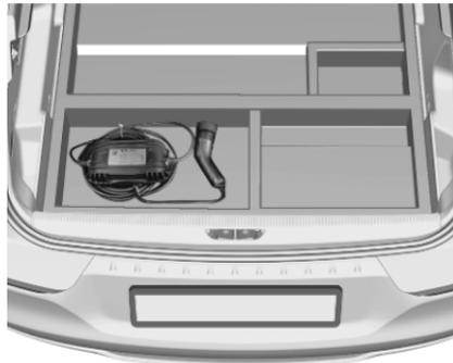
A portable charging cable used to charge the vehicle high voltage battery is stored under the rear floor storage cover in the load compartment ⇨ 191. The charging cable is compatible with the domestic
