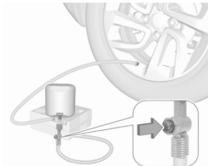
Drain excess tyre pressure with the button on the air hose.
