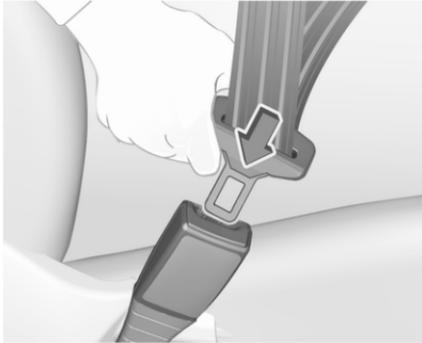
Loose or bulky clothing prevents the seat belt from fitting snugly. Do not place objects such as handbags or mobile phones between the seat belt and your body.
