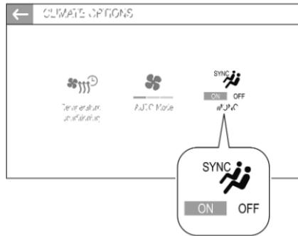
Set **SYNC** to **ON** to link passenger side temperature setting to the driver side. Touch **MONO** or **SYNC** to link passenger side temperature setting to the driver side.
