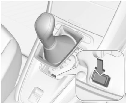
3. Push down the button and move the selector lever out of **P**. Have the cause of the power supply interruption remedied by a workshop.
