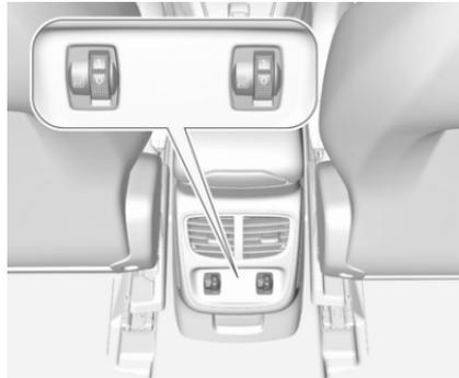
Adjust seat heating by turning thumb wheel
