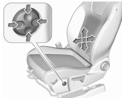
Adjust lumbar support using the four-way switch to suit personal requirements.
