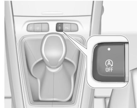
Deactivate the stop-start system manually by pressing
