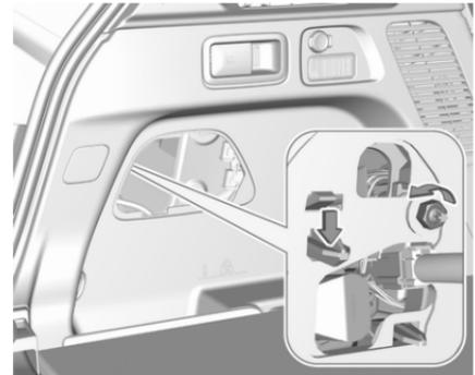
2. Slacken the light fixing nut using a box spanner or socket.
