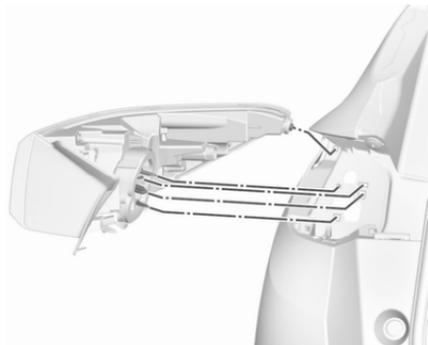
5. From the outside, carefully withdraw the light assembly from recess and remove. Take care that the cable duct remains in position.
