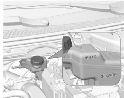
The brake fluid level must be between the **DANGER** and **MAX** marks.
