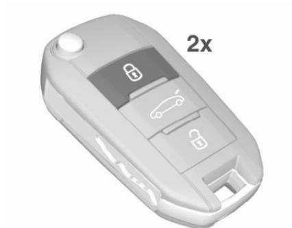
Press Ⓛ on the radio remote control twice within 5 seconds.
