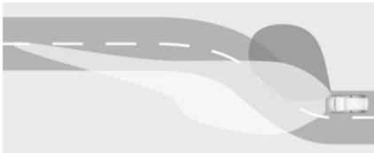
Particular LEDs, based on steering angle and speed, are additionally triggered to improve lighting in curves. This function is activated at speeds from 25 mph to 43 mph.
