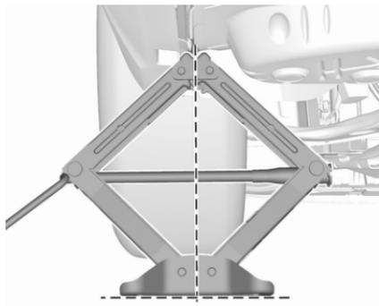
4. Set the jack to the necessary height. Position it directly below
