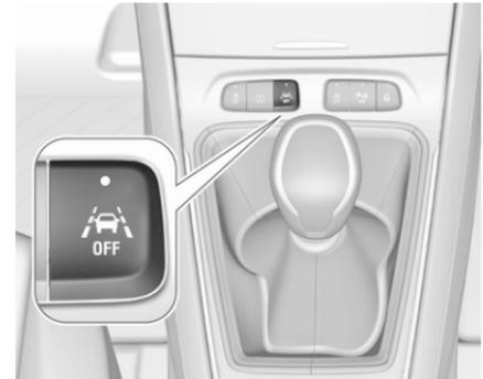
If the system is activated, the LED in the button
