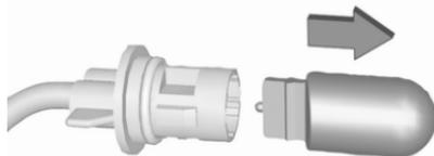
3. Detach the bulb from the bulb socket and replace the bulb.
