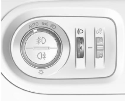
To adapt headlight range to the vehicle load to prevent dazzling, turn thumb wheel
