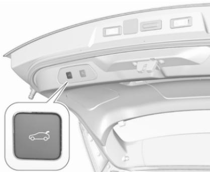
3. Press and hold the button
