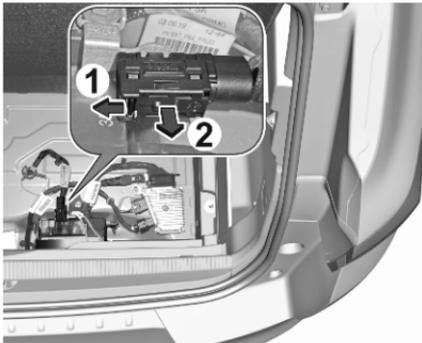
4. Push (1) the unlock lever and remove (2) the lead from the connection pin.
