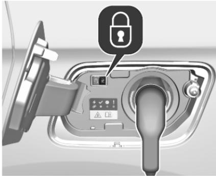
Once charging, the vehicle plug will be locked to the charging port and cannot be disconnected while charging is active.
