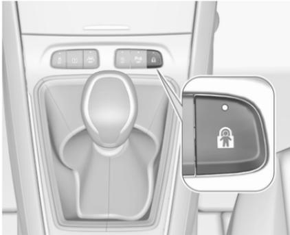
Remotely operated system to prevent opening of the rear doors via the interior door handles and the use of the rear power windows.
