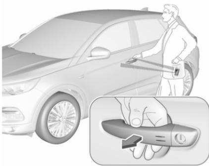
The electronic key must be outside the vehicle, within a range of approx. 1 m of the relevant door side.
