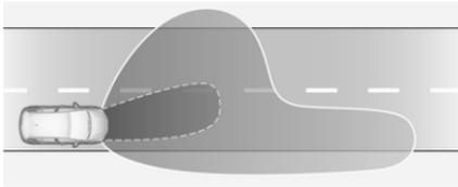
Controlled by wiper or rain sensor. The wide light distribution – slightly swiveled to the outside – enables improved orientation at the edge of the road. The intensity of the light in the far distance is increased in order to recognise objects and markings on the right road side and obstacles on the lane despite the weather condition. By lowering the reflection on wet roads the oncoming traffic is less dazzled. Adverse weather light is activated up to a speed to 43 mph.
