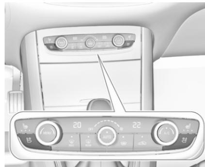
Activate ventilation by pressing for the respective front seat.
