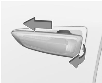
1. Slide the light assembly forward and remove it at the back.
