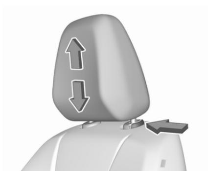
Press release button, adjust height, engage.
