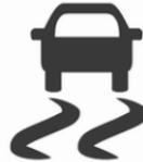
ESC and traction control system are operational after each engine start as soon as the control indicator
