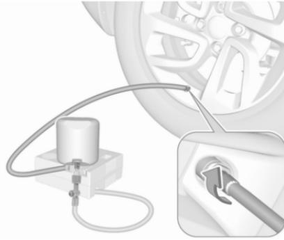
7. Screw the filler hose to the tyre valve.
