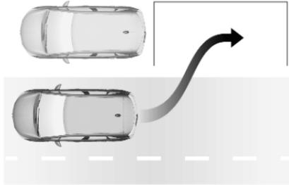
Move forwards and backwards while observing the warnings of the parking assist until the end of manoeuvre is indicated.
