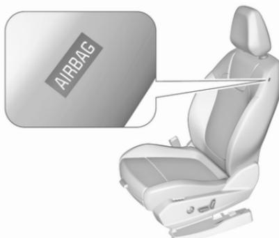
The side airbag system consists of an airbag in each front seat backrest. This can be identified by the word **AIRBAG**.
