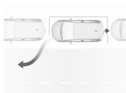
Move forwards and backwards while observing the warnings of the Parking assist until the end of manoeuvre is indicated. The manoeuvre is complete when the vehicle's front wheels are out of the parking slot.
