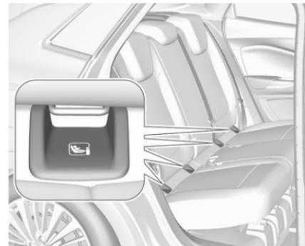
Fasten vehicle-approved ISOFIX child restraint systems to the ISOFIX brackets. Specific vehicle ISOFIX child restraint system positions are marked in the ISOFIX table ⇨ 64.
