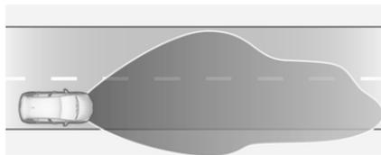
Activated automatically at a speed above 71 mph. Illumination is adapted to the higher speed driven on motorways. If there is no oncoming traffic, the visibility on the side of the vehicle is increased. The visibility range raises from 70 m to 140 m allowing distant objects to be recognised across the entire width of the road.
