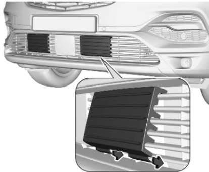
2. Press the lower part of the protection cover against the slat of the grille. Ensure that the protection cover is fixed securely.
