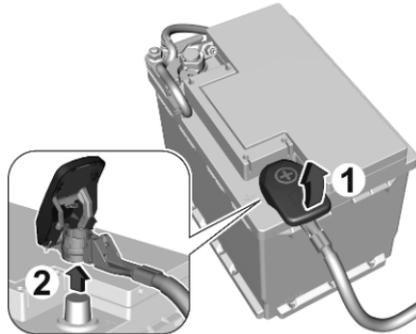
2. Pull (1) the lever of the clamp of the positive (+) terminal upwards and remove (2) the clamp from the terminal.
