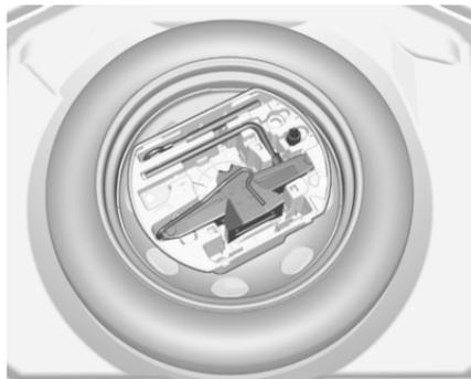
The jack, the towing eye, chocks and the tools are located in the tool box.
