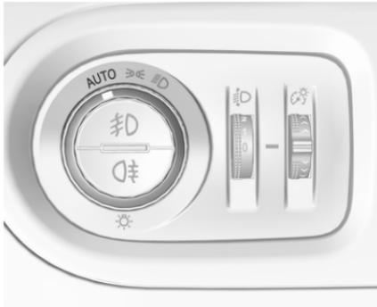
When the automatic light control function is switched on and the engine is running, the system switches between daytime running lights and headlights automatically depending on the external lighting conditions and information given by the wiper system.
