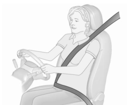
Pull out the seat belt and fasten in seat belt buckle. The seat belt must not be twisted and must fit close against the body. The backrest must not be tilted back too far (maximum approx. 25°).
