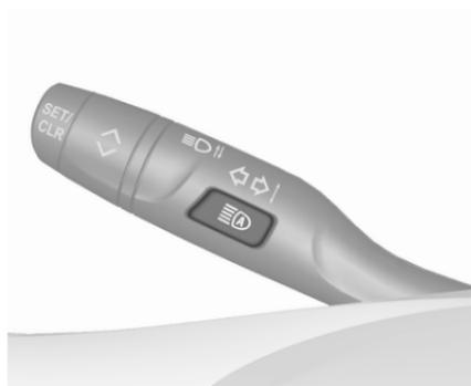
Activate the high beam assist by pressing
