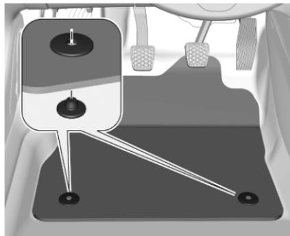
2. Align slots in the mat with the retainers, as shown.
