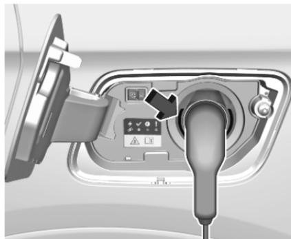
The start of charging is indicated by the green flashing of the status indicator at the charging port and at the control box of the charging cable.
