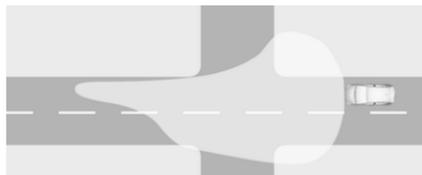
Activated automatically at a speed up to approx. 34 mph and in situations with exterior ambient light. The light is wide and symmetrical. If the speed is below 19 mph, the headlamps are slightly swiveled to the outside to allow an earlier recognition of pedestrians and objects on each side of the road. A special beam pattern is designed to avoid glare for other road users.
