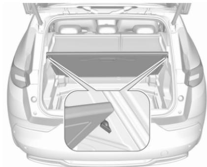
To hold the load compartment cover in an upright position, lift it up past the retractable stops.
