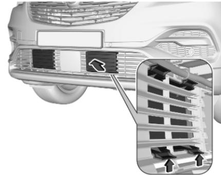
1. With your hand behind the grille, push the brackets of the protection cover upwards to release the protection cover.
