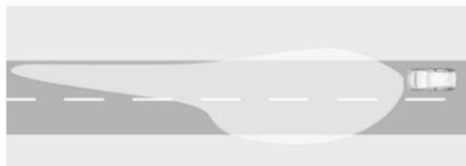
Activated automatically at a speed between 34 mph and 71 mph when driving in rural areas. The illumination
