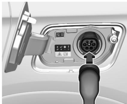
5. Plug in the vehicle plug of the charging cable into the charging port on the vehicle.
