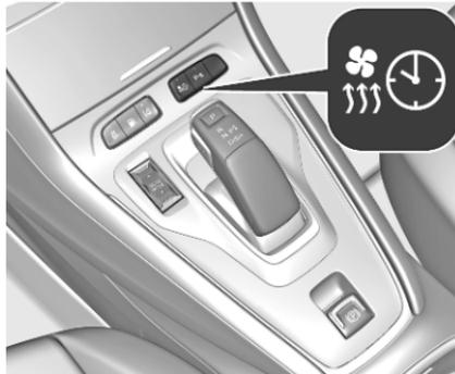
The operating status of the parking heater is shown by a LED.
