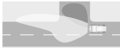
Activated at a speed of up to 25 mph when turning off. The light consists of particular LEDs which illuminate the direction of travel. These LEDs are triggered depending on the steering angle or the activation of the turn lights.
