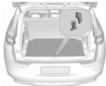
The rear floor cover can be lifted and removed. Raise cover at the loop and remove.
