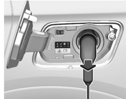
2. Disconnect the vehicle plug from the charging port within 30 seconds.
