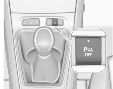
The system is switched off when reverse gear is disengaged. Press
