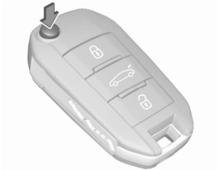
Press button to extend. To fold the key, first press the button.
