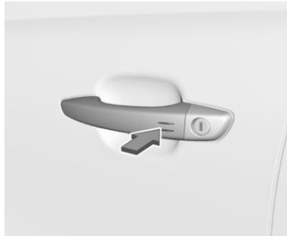
Electronic key system: Unlocking the vehicle by pressing on one of the front door handles at the markings deactivates the anti-theft alarm system.
