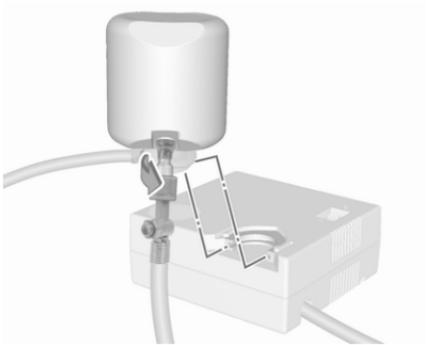
4. Screw the compressor air hose to the connection on the sealant bottle.
