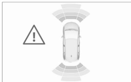
Additionally, the distance to rear and front obstacles is displayed by changing distance lines in the Info Display ↻ 100.
