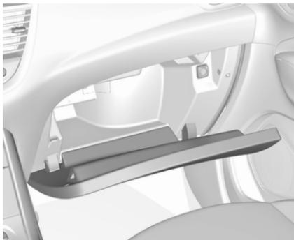
On some versions the glovebox is ventilated. Air ventilation and temperature depend on the settings of the climate control system. The air vent in the glovebox can be closed ⇨ 128.
