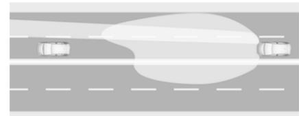
If the vehicle is equipped with uplevel-LED headlights, high beam assist includes a special motorway mode. When driving faster than 71 mph on motorways, the light beam becomes smaller to avoid dazzling of oncoming traffic. When following vehicles ahead or passing, dazzling for these vehicles is reduced.
