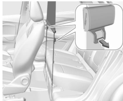
Pull the flap at the tightener on both sides to release the straps. Detach hooks from the loops.
