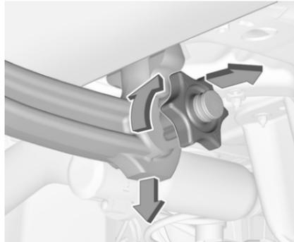
Open the protective flap and turn the key to position
