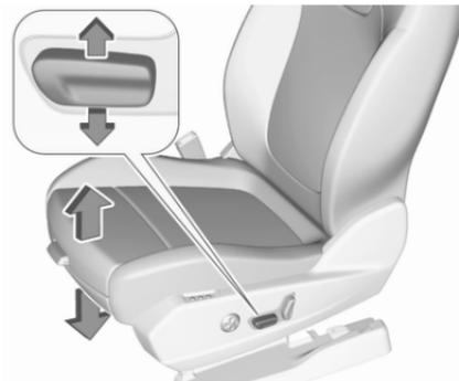
Move switch upwards / downwards.
