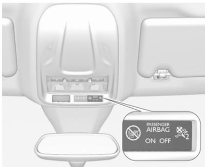
If the control indicator
