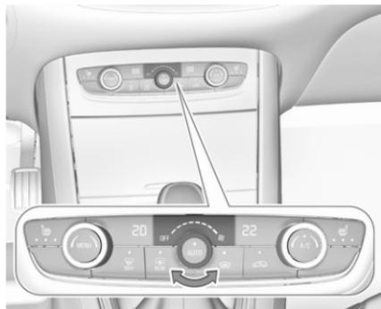
Adjust the air flow by turning rotary ring to the desired speed. Turn anticlockwise to decrease or turn clockwise to increase. Fan speed can also be changed in the climate control settings menu. Press **MENU** to enter the climate control settings menu.
