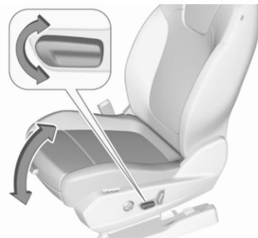
Move front of switch upwards / downwards.
