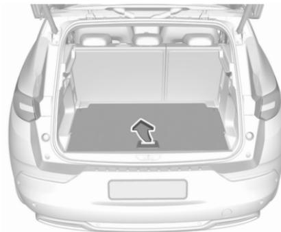
To remove, press the handle to unlock the load floor and lift it up while using the handle.
