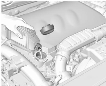
The engine oil level must not exceed the **MAX** mark on the dipstick.
