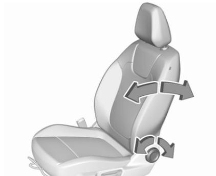
Turn handwheel. Do not lean on backrest when adjusting.
