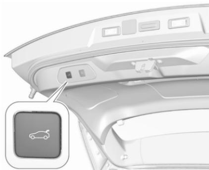
To close, press
