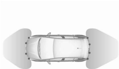
The system operates with ultrasonic parking sensors in the rear and front bumper.
