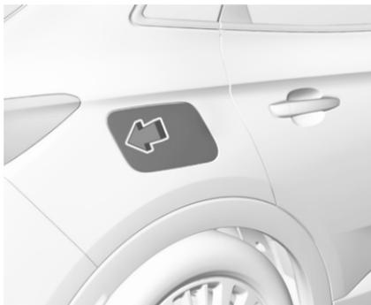
The fuel filler flap can only be opened if the vehicle is unlocked. Open the fuel filler flap by pushing the flap.
