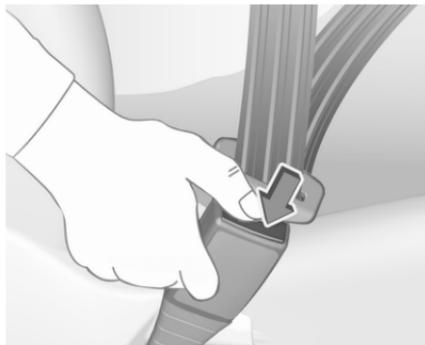
To release seat belt, press red button on seat belt buckle.
