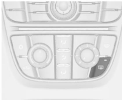
The heating is operated by pressing the
