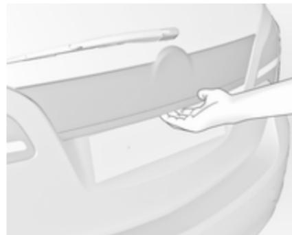
After unlocking, push the touchpad switch under the tailgate moulding and open the tailgate.
