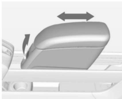
Pull the front handle slightly and move the armrest to the desired position. Release the handle. Move the armrest until it engages audibly.
