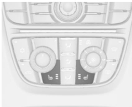
Adjust heating to the desired setting by pressing the
