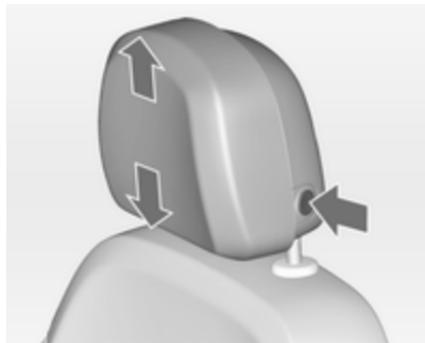
Press release button, adjust height and engage.
