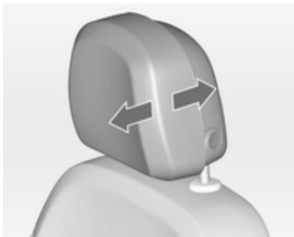
To adjust horizontally, pull the head restraint forwards. It engages in several positions.
