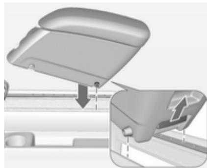
Press the rear button and insert the rear guide pins into the upper guide rails. Release the button.
