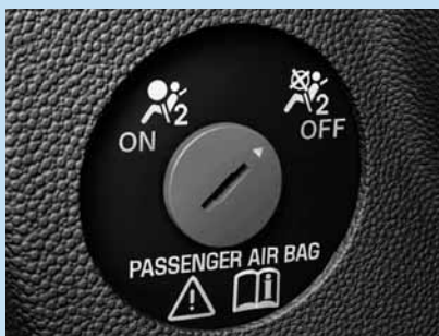
Deactivation for front passenger's airbags.
