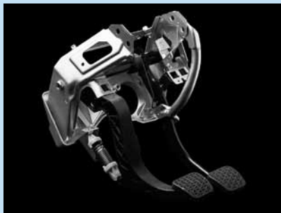
Pedal release system.
