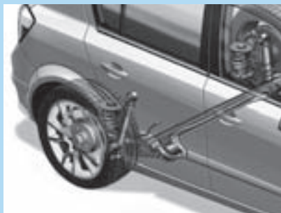
Lightweight torsion beam rear axle.
