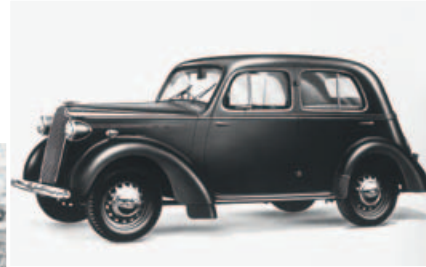
1937 – The Vauxhall 'H'-type, the first British car to have integral construction.
