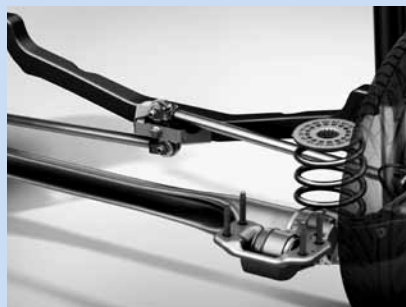
Watt's link improves handling and ride comfort.
