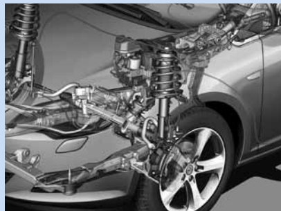
MacPherson strut front suspension.
