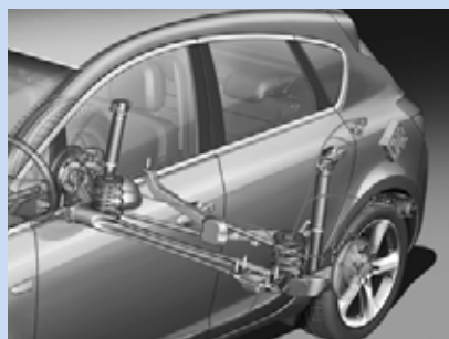
Compound crank rear suspension includes innovative use of Watt's link
