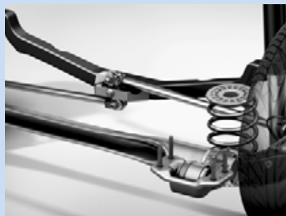
Watt's link improves handling and ride comfort.
