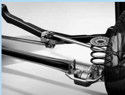
Watt's link improves handling and ride comfort.
