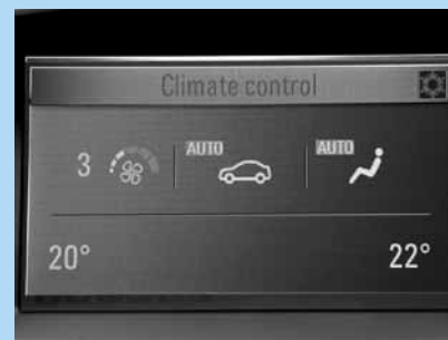
Dual-zone Electronic Climate Control (ECC).
