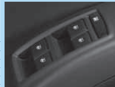
Electrically operated windows.
