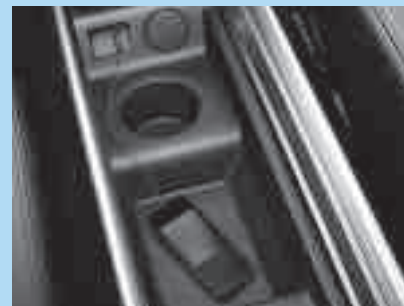
Auxiliary-in socket and USB connection.
