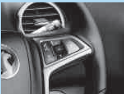
Steering wheel mounted audio controls.
