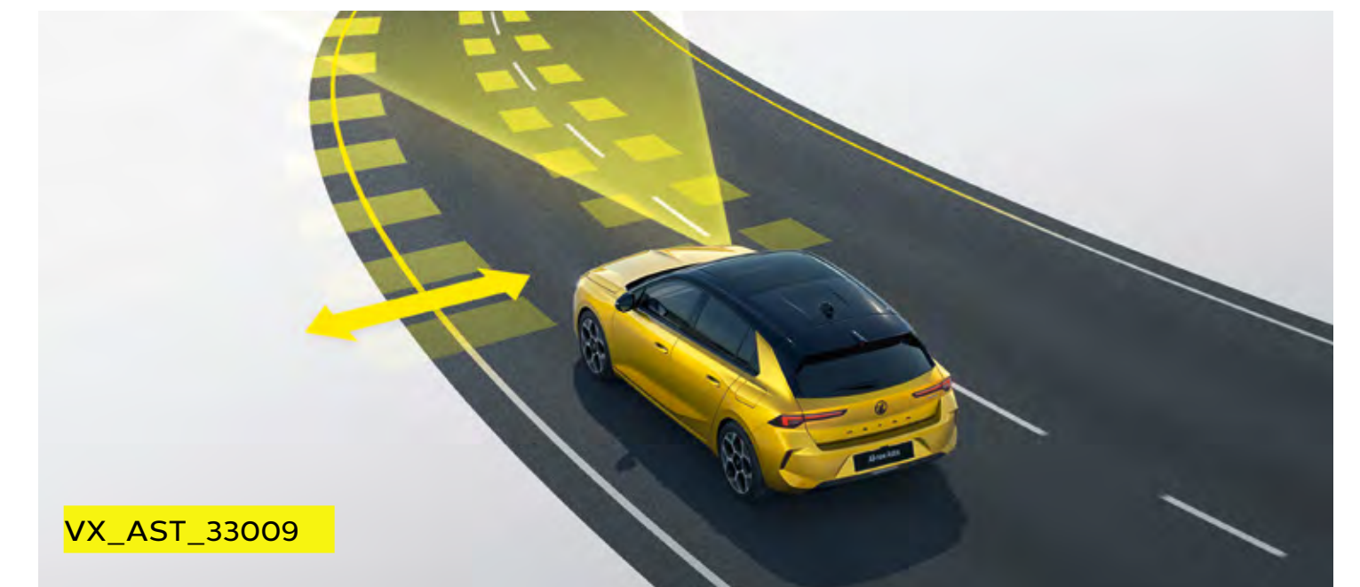
Lane departure warning with lane keep assist.
