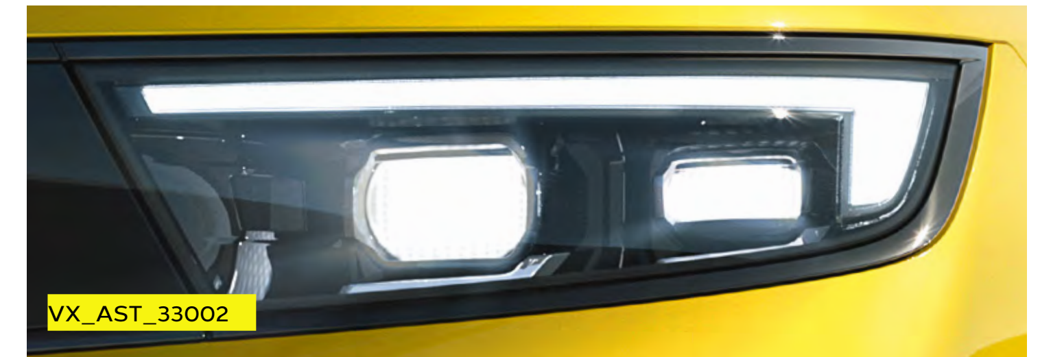
IntelliLux adaptive LED® pixel headlights.
