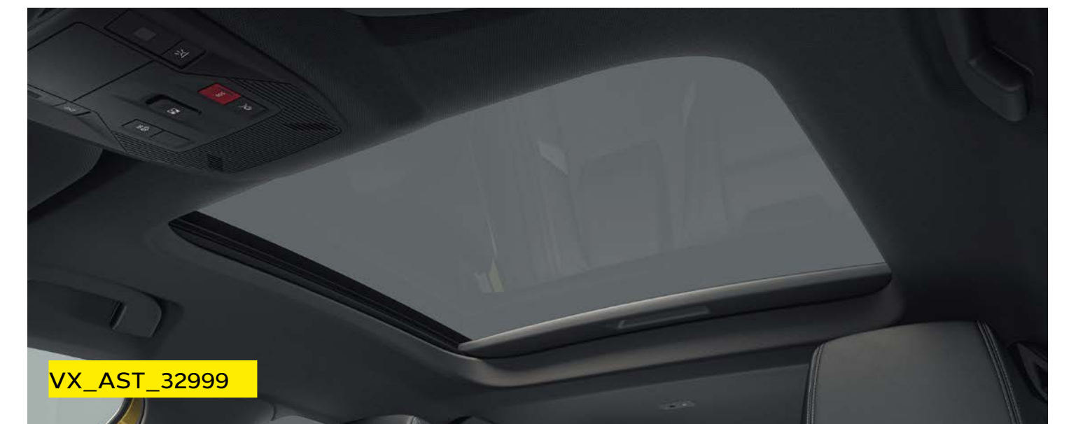
Electrically operated slide/tilt glass sunroof with blind.
